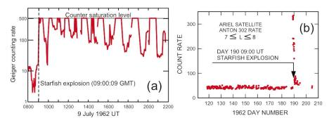
**Fig. 23** (a) The Geiger counting rate observed on the Ariel-1 satellite. In the hours following the explosion the instrument regularly saturated on each orbit as the spacecraft crossed the forming artificial radiation belt. (b) In the long term observations of the stable high energy cosmic rays by Ariel-1, the high energy electrons injected by the explosion stand out even at high value L-shells. [Figures from Durney et al. (1962) and Elliot (1966).]
