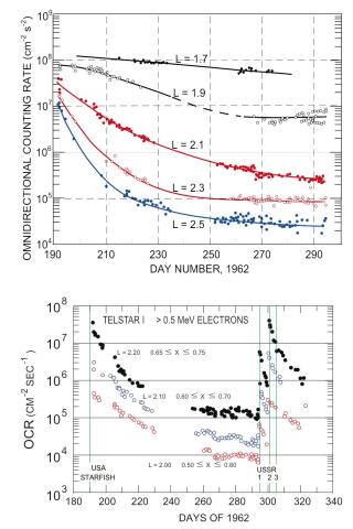
sions). The new population, superimposed on the decaying Starfish belt, is well illustrated in Fig. 15 (from Brown, 1966). The peak intensities appeared close to that from Starfish; the decay constants appeared to be quite comparable to those experienced by the Starfish fluxes.
