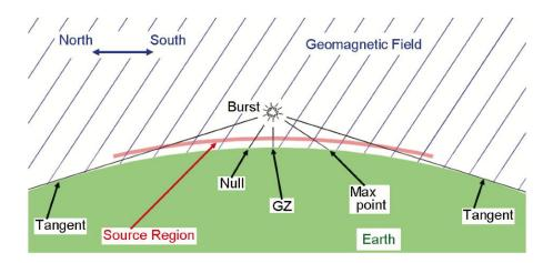
**Fig. 6** Typical geometry of E1 phase. There are three special points on the ground: Ground Zero (GZ) – is the point directly below the burst, Null Point – where the observer ray and geomagnetic field lines are parallel, and Max Point – where the E1 HEMP has its maximum peak level (from Savage et al., 2010).
