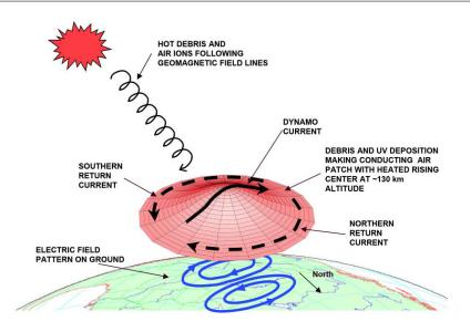
Fig. 9 Schematic of E3B Heave phenomenology (from Gilbert et al., 2010).
