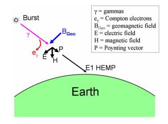
Longmire (1986) explains the basic physics of the E1 pulse in terms of an oversimplified "flat Earth" scenario. While this scenario is clearly unphysical, it clarifies the basic physics and explains the extremely short duration of the initial pulse. Here we briefly outline his derivation.
