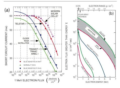
**Fig. 26** (a) Solar cell damage curves. Based on Figure 3 in Rosenzweig et al. (1963) and Figure 8 in Hess (1963). The performance of the modern solar cells is taken from Xin et al. (2014). (b) Natural and artificial energetic electron fluxes showing cumulative spectra above 40 keV. From Fig. 4 in Wenaas (1978).
