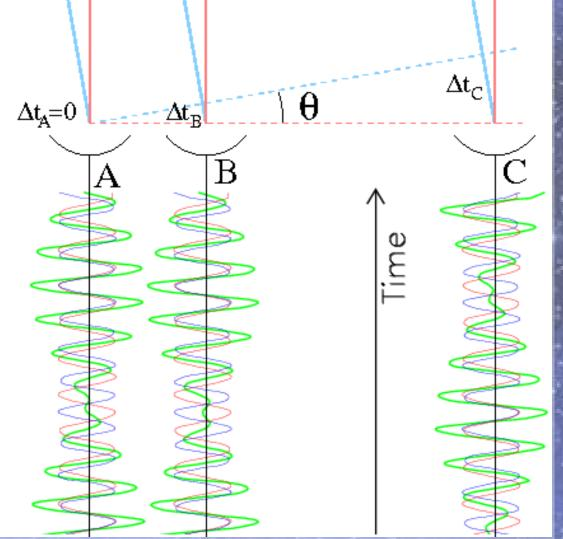
Figure 9: Telescopes A and B being close together receive beats almost at the same time resulting in a high degree of correlation. Telescopes A and C being further apart, do not receive beats at the same time and the correlation is low.
