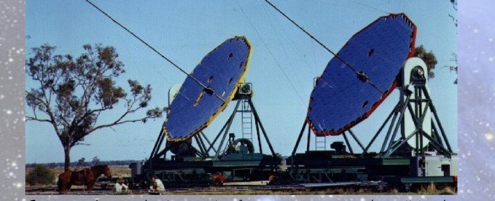
Figure 8: The Narrabri Intensity Interferometer was constructed in 1965 and operated until 1971. Each telescope was 6m in diameter, twice as large as the StarBase telescopes.
