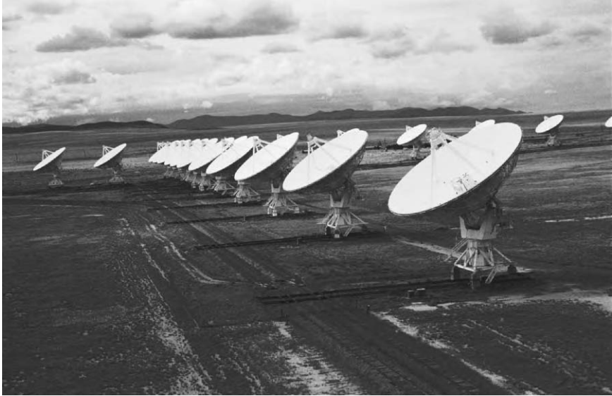
FIGURE 1.3. The VLA radio telescope of the National Radio Astronomy Observatory located west of Socorro, NM, out in the middle of nowhere, which is the way radio astronomers like it. In this view many of the dishes are spaced in the so-called compact array. The railroad tracks on which the dishes can be moved for up to 11 miles along each of three arms of the array can be seen in the foreground. (Image courtesy of NRAO/AUI.)
