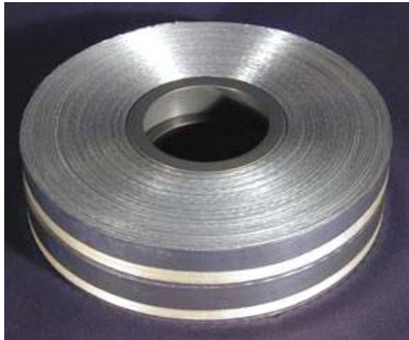
Figure 5. Two Stacked Dual-200-m Windings
