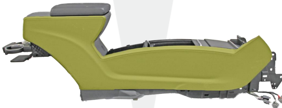
Figure 26 (RH center console closeout panel highlighted)
