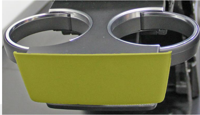
Figure 17 (Rear cup holder trim panel highlighted)
