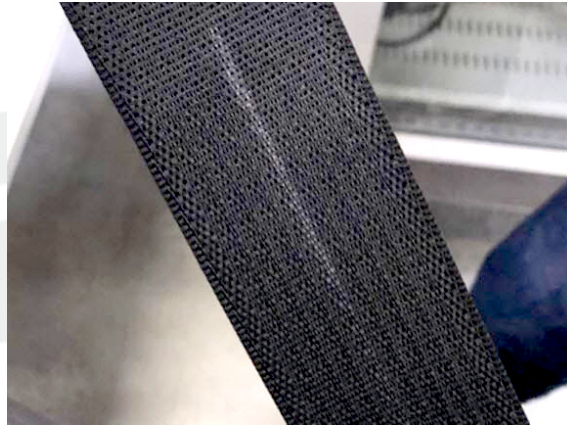
Figure 8 (Mark caused by bolt rubbing on belt)
