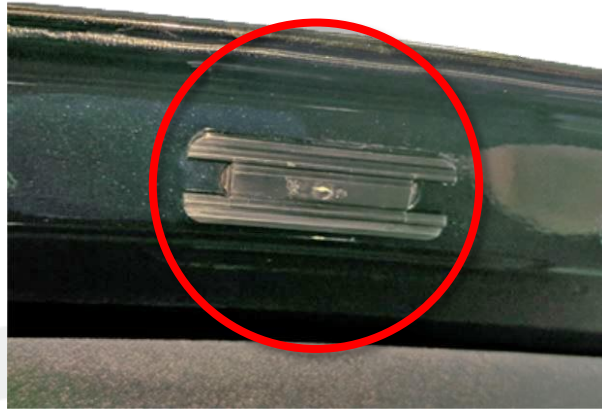
Figure 2 (Updated drain-type LH liftgate plug installed, RH similar)
