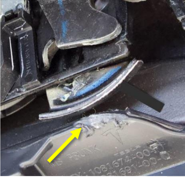
Figure 1 (Underhood storage unit damaged)
