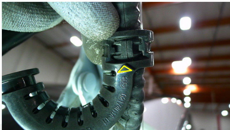
Figure 5 – Align arrow on grommet support with slot in rubber armor
