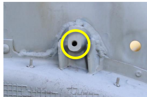
✓ Figure 4 (2nd row lower seat belt hole in 1 st generation rear node)
