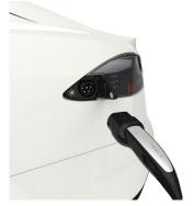
5. When you plug the Mobile Connector into your vehicle, a light around the charge port pulses green during charging and the instrument panel displays charging information.
