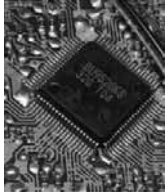
FIGURE 1.20 A packaged IC soldered onto a printed circuit board.
