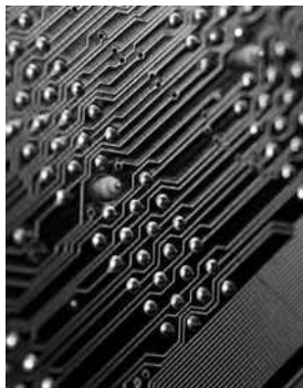
FIGURE 6.19 A through-hole PCB.
