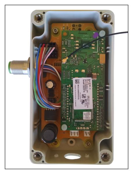
The following photo shows an industrial IoT device that uses a cellular modem:
