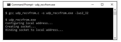
You could use udp\_client to connect to udp\_recvfrom for testing, or you can implement udp\_sendto, which we will do next.
