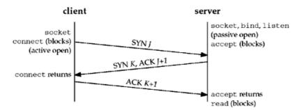
Figure 2.2. TCP three-way handshake.
