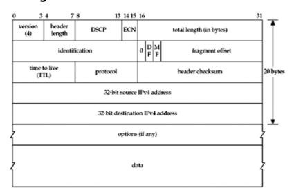
Figure A.1. Format of the IPv4 header.
