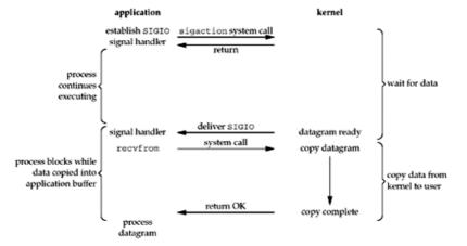
Figure 6.4. Signal-Driven I/O model.
