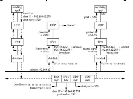
Figure 20.4. Example of a broadcast UDP datagram.
