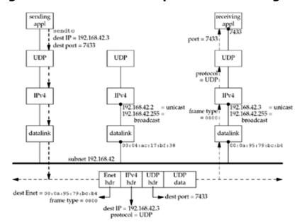
Figure 20.3. Unicast example of a UDP datagram.
