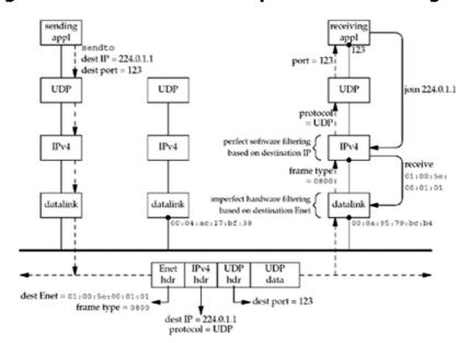
Figure 21.4. Multicast example of a UDP datagram.
