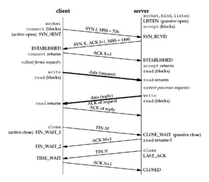
Figure 2.5. Packet exchange for TCP connection.
