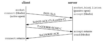
Figure 2.6. SCTP four-way handshake.
