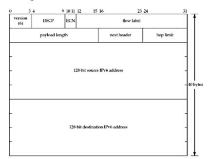
Figure A.2. Format of the IPv6 header.
