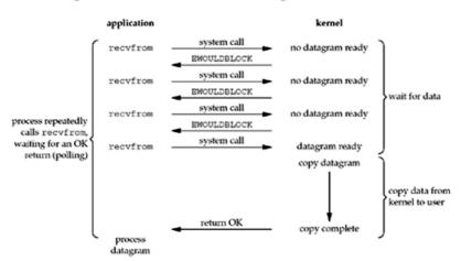
Figure 6.2. Nonblocking I/O model.
