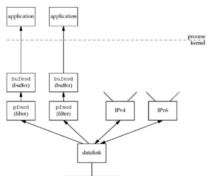
Figure 29.2. Packet capture using DLPI, pfmod, and bufmod.
