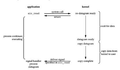
Figure 6.5. Asynchronous I/O model.
