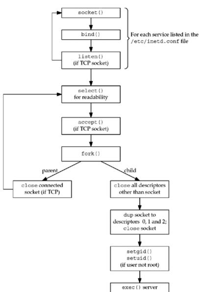
Figure 13.7. Steps performed by inetd.
