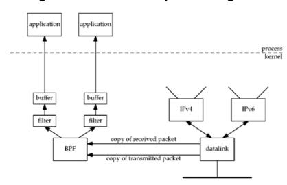
Figure 29.1. Packet capture using BPF.
