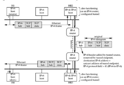
Figure B.2. IPv6-in-IPv4 encapsulation on 6bone.
