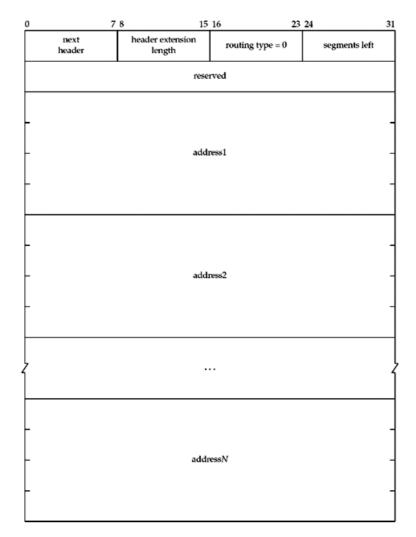
Figure 27.11. IPv6 routing header.
