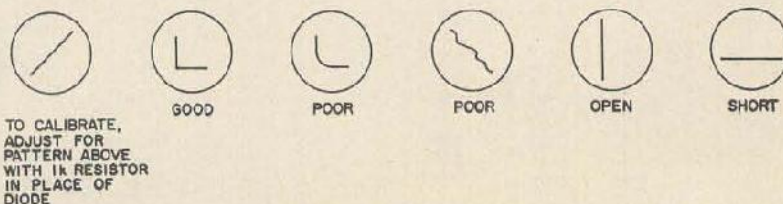
Fig. 112. One of the easiest types of diode checks for a person with a scope is this, but it tells nothing about a diode's high voltage performance.
