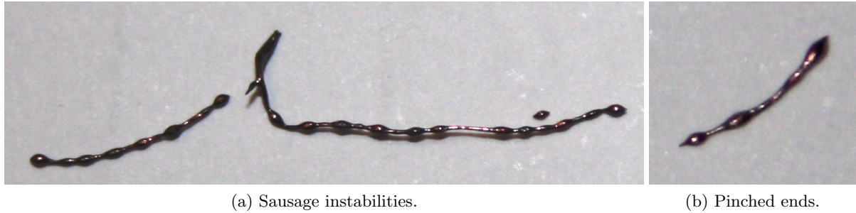
Figure 4.4 Fragments of wire show signs of sausage instabilities caused by MHD forces, eventually causing fragmentation when the copper is liquid. \ell = 6 m, d = 0.2 mm, V_0 = 10.5 kV, E_0 = 1.75 kV/m.
