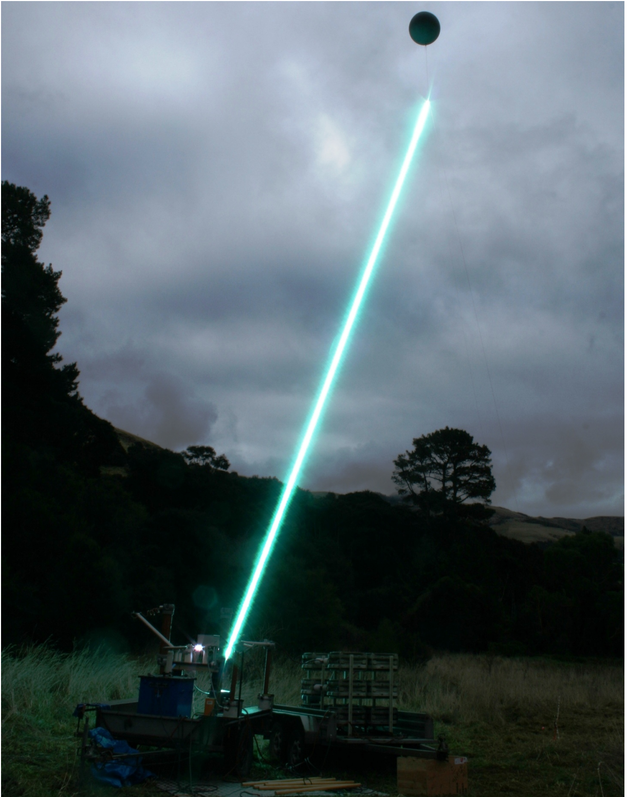
Figure 6.12 A 15 m restrike produced by an EW that was suspended from a helium-filled weather balloon. The 0.63 mm diameter return wire was also suspended from the balloon. \ell = 15 m, d = 0.2 mm, V_0 = 90 kV, E_0 = 6 kV/m.
