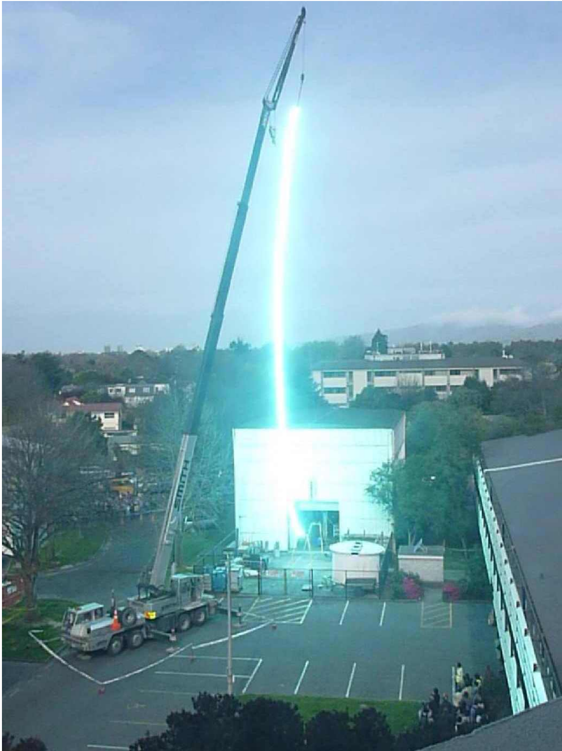
Figure 6.5 A 36 m vertical restrike produced with an EW suspended from a crane as part of a demonstration. Public observers can be seen in the foreground and also behind the laboratory. A weather observer at the University mistook the experiment for ‘dry-day lightning’. \ell = 36 m, d = 0.2 mm, V_0 = 180 kV, E_0 = 5 kV/m. Photo credit: Philippa Martin.
