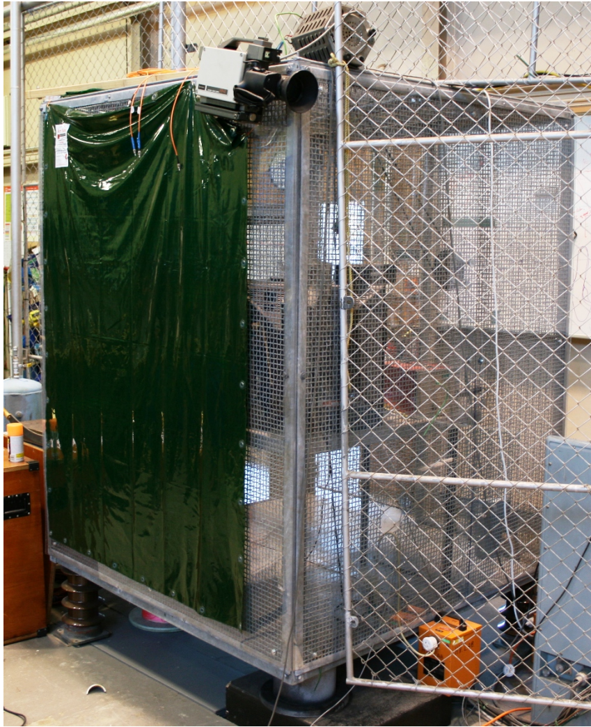
Figure 3.22 The Faraday cage, covered with 5 mm thick polycarbonate. A green welding screen covers one wall. The VariAC can be seen on the top of the cage, and the video camera for viewing the charging instrumentation is seen on the side.
