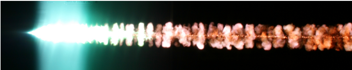
Figure 4.16 A streak photograph, using the short-exposure technique, of a wire that produced restrike. The camera was rotated 90^\circ such that the camera shutters move along the axis of the wire. Time increases from left to right in this photograph. Approximately 2 ms of time is represented. \ell = 3 m, d = 0.2 mm, V_0 = 25 kV, E_0 = 8.3 kV/m.
