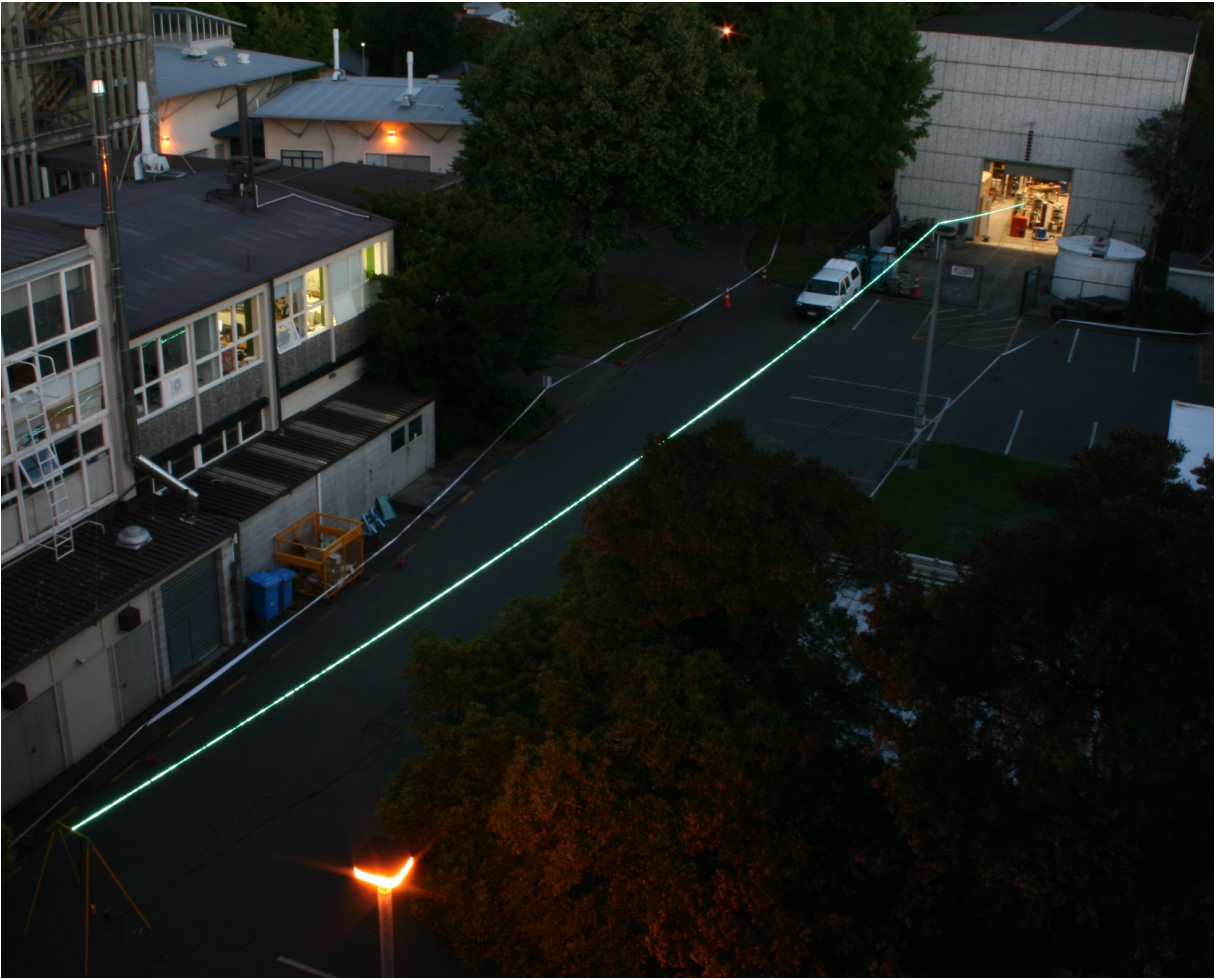
Figure 6.6 A 60 m experiment outside the high voltage laboratory that did not produce restrike. The plasma beads were very close to forming a continuous plasma column. A tree was obscuring the a short section of the wire in the middle of the image. \ell = 60 m, d = 0.2 mm, V_0 = 270 kV, E_0 = 4.5 kV/m. Photo credit: Ryan van Herel and Stewart Hardie.
