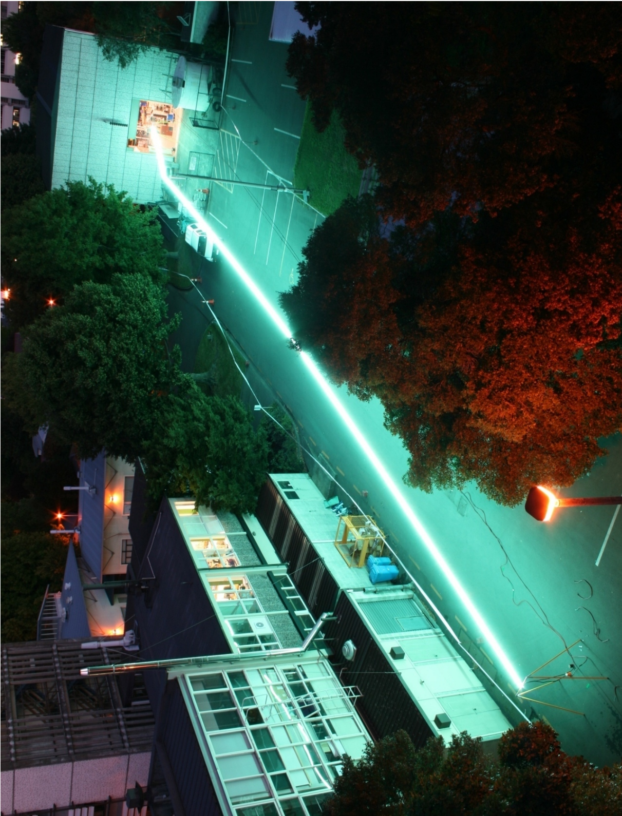
Figure 6.7 A 60 m restrike outside the high voltage laboratory. \ell = 60 m, d = 0.2 mm, V_0 = 285 kV, E_0 = 4.75 kV/m. Photo credit: Ryan van Herel and Stewart Hardie.
