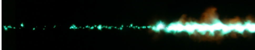
(b) Left: \ell = 0.7 m, d = 0.26 mm EW forms plasma beads; Right: \ell = 1.3 m, d = 0.25 mm EW produces restrike. V_0 = 18 kV.
