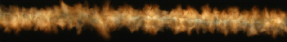
(b) \ell = 2 m, d = 0.2 mm, V_0 = 45 kV, E_0 = 22.5 kV/m
