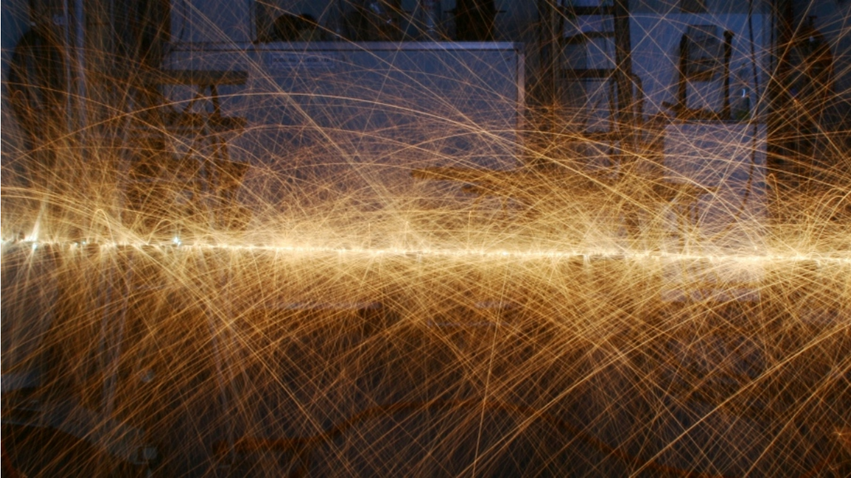
(a) Liquid copper droplets ejected from a wire.
