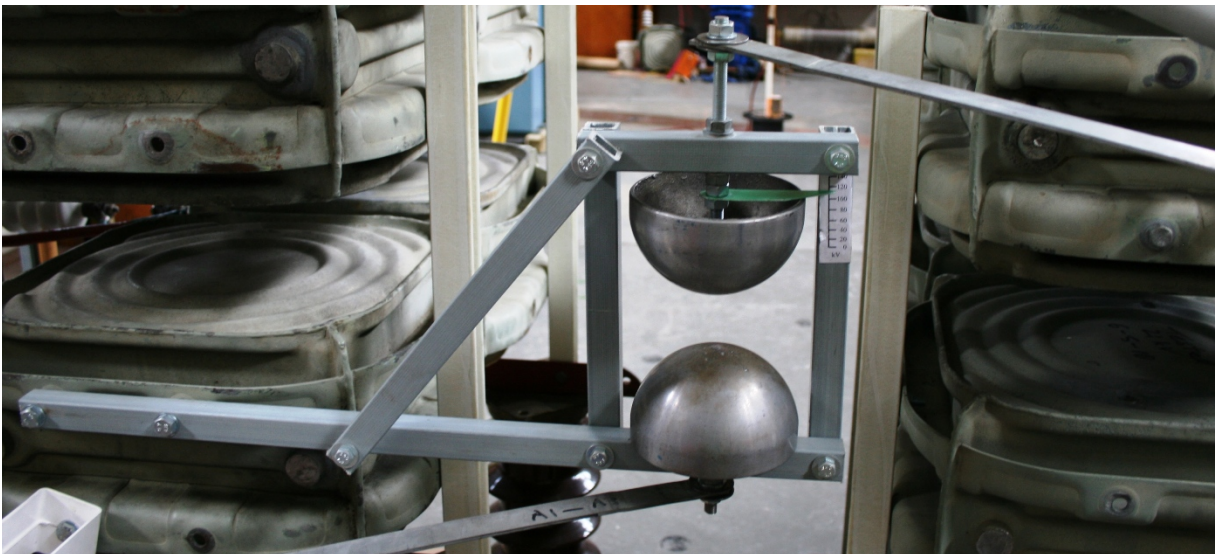
Figure 3.15 Spark gap S_2 . The top hemisphere was connected to C_2 and the bottom hemisphere was connected to C_3 . An adjustment scale with a green pointer can be seen to the right of the top hemisphere.
