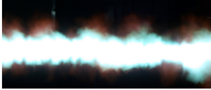
Figure 4.20 A long-exposure photograph of an experiment in Region IV. \ell = 1 m, d = 0.2 mm, V_0 = 35 kV, E_0 = 35 kV/m.
