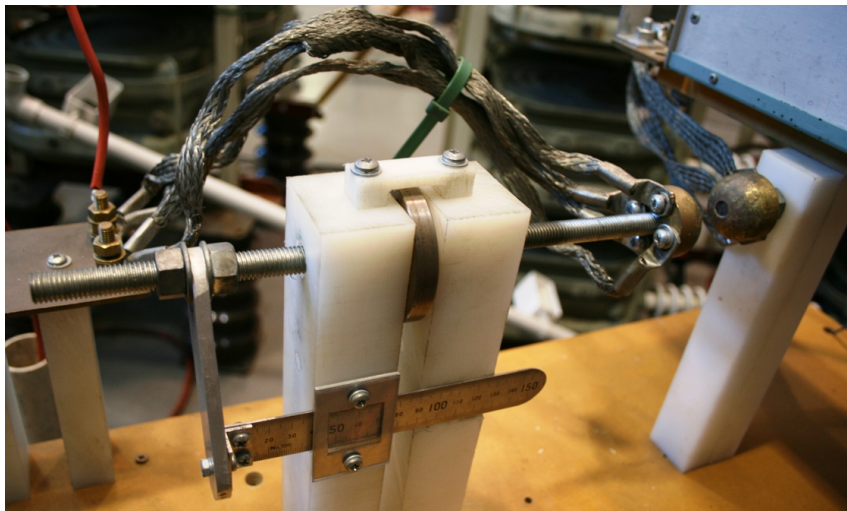
(b) Detail of the main gap, adjustment nut and gap length indicator.
