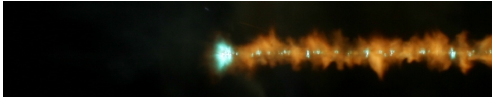
(a) Left: \ell = 0.7 m, d = 0.26 mm EW remains intact; Right: \ell = 1.3 m, d = 0.25 mm EW forms plasma beads. V_0 = 30 kV.
