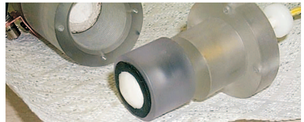
Fig. 11. Photographs of the TTU ferroelectric generator (courtesy of Texas Tech University).
