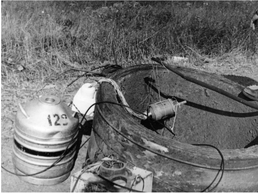
Fig. 23. Superconducting generator (Courtesy of A.B. Prishchepenko).
