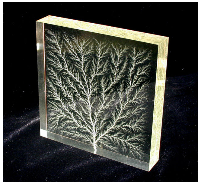
Fig. 5: Treeing in a block of Plexiglas. © Bert Hickman
