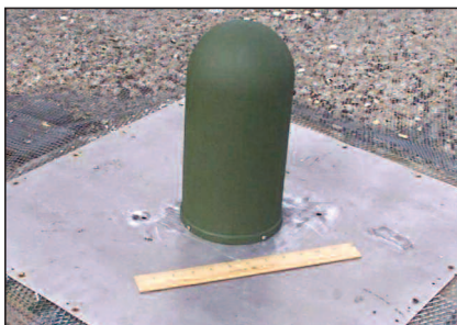
▲ Fig. 14 Complete TASH 225 to 2000 MHz prototype on an outdoor ground plane.
