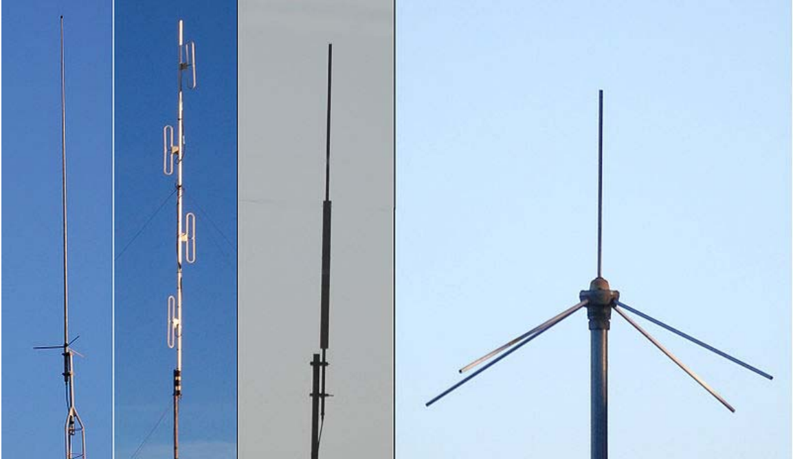
Examples of US 136-174 MHz base station antennas.
