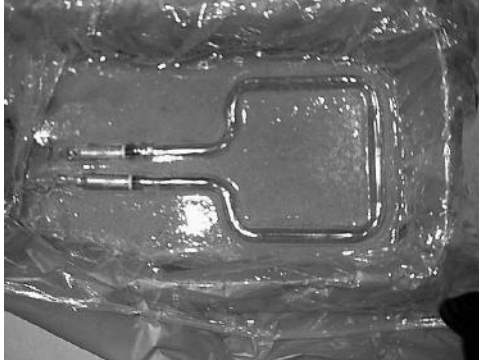
Figure 9.35 Embedded plasma antenna in a sandstone epoxy slurry that solidified. Note that the reflection of light from the glass tube containing the plasma gives a metallic appearance but it is glass.
