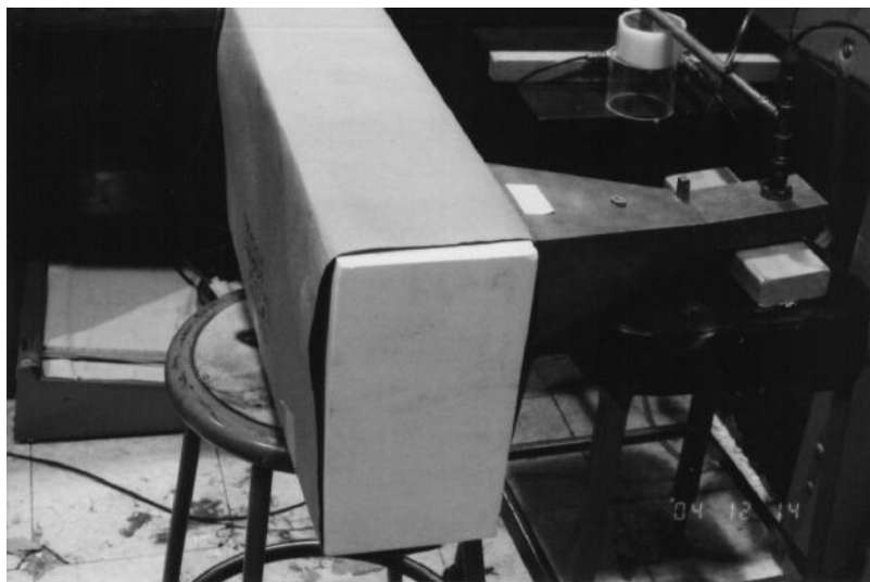
Figure 9.37 Setup of SynFoam to measure the index of refraction by measuring the phase shift.
