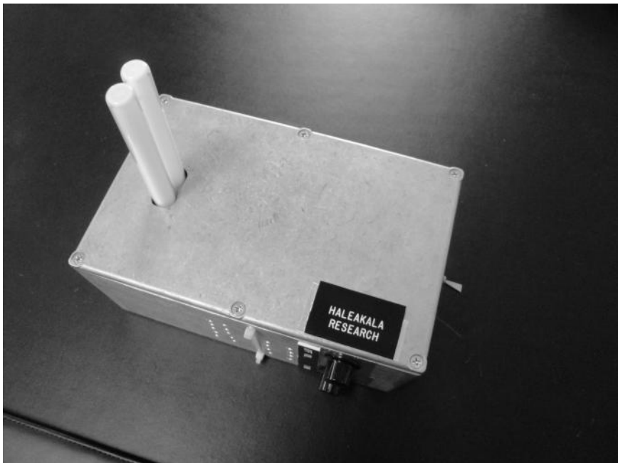
Figure 4.4 This plasma antenna has no external wires other than the one going to the charger. Once the battery is charged, the charger cable should be unplugged, leaving a self-contained plasma antenna with minimal interference from stray signals.
