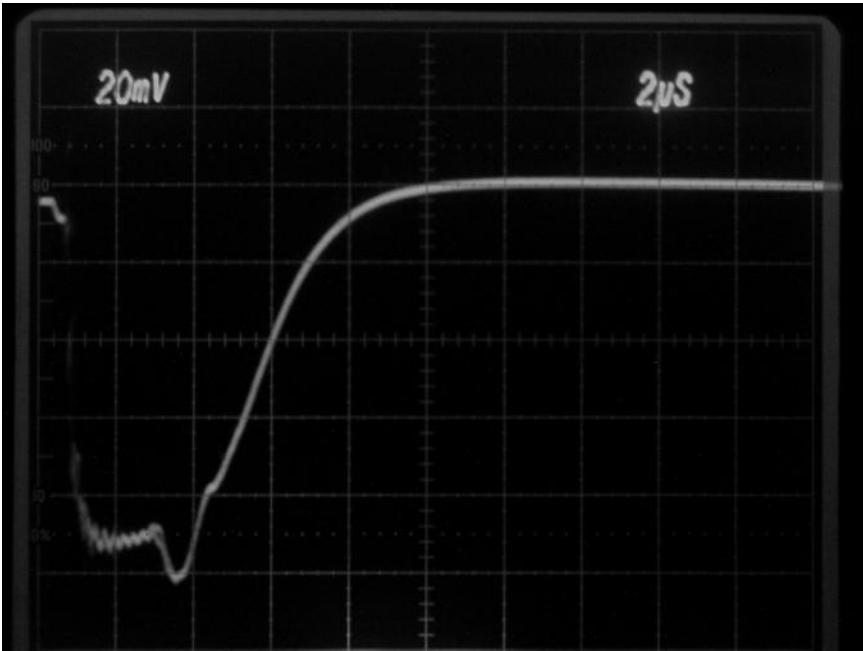
Figure 9.34 Reflection experiments at 80 mTorr. The pressure is different from the pressure used for measurements as shown in the other figures in the set (Figures 9.29–9.34), but other conditions and scales are the same. A resonance (the dip shows an increased reflection) is observed at this pressure and is less pronounced than the resonance at 380 mTorr.
