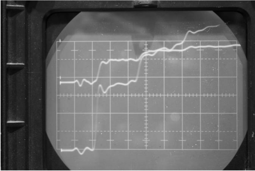
Figure 9.26 The potentiometer replaced by the 75-ohm line.
