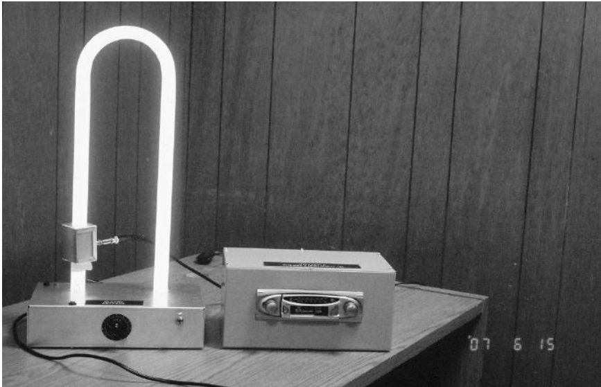
Figure 4.1 Plasma antenna using a standard U-shape fluorescent lamp and ballast. A variable voltage transformer (Variac) controls plasma current and density. An FM receiver is in the box on the right with a coaxial cable connected to a capacitive coupler surrounding the fluorescent lamp (on the left side of the lamp).
