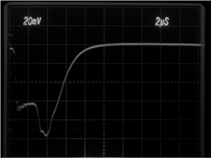
Figure 9.33 Reflection experiments at 380 mTorr. The pressure is different from the pressure used for measurements as shown in the other figures in the set (Figures 9.29–9.34), but other conditions and scales are the same. A resonance (the dip shows increased reflection) is observed at this pressure and is more pronounced than the resonance at 1.1 Torr.
