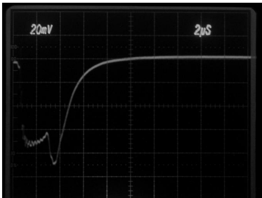
Figure 9.32 Reflection experiments at 1.1 Torr. The pressure is different from the pressure used for measurements as shown in the other figures in the set (Figures 9.29–9.34), but other conditions and scales are the same. A resonance (dip shows increased reflection) is observed at this pressure and is more pronounced than the resonance at 2.0 Torr.
