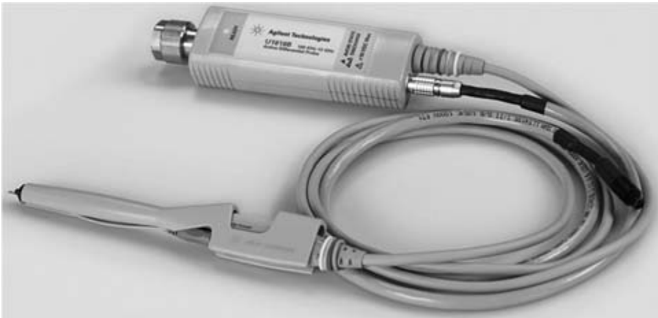
Figure 12-5 An active probe is designed with an amplifier having very low input capacitance so that wide bandwidth signals can be probed with minimal loading. (© Keysight Technologies, Inc. Reproduced with Permission, Courtesy of Keysight Technologies, Inc.)
