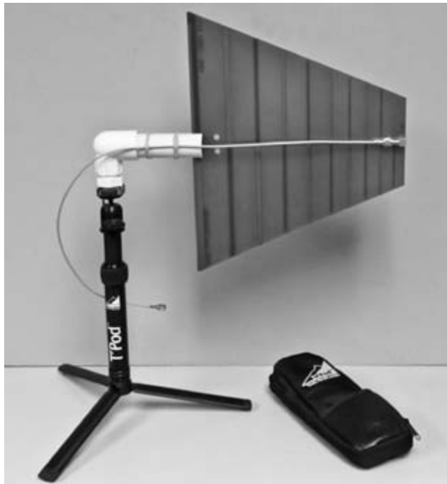
Figure 16-13 This 400–1000 MHz log periodic antenna is usable for troubleshooting purposes down to 100 MHz. The antenna is fashioned from PC board material (available from http://wa5vjb.com ) and mounted on a simple tripod. (Courtesy Kenneth Wyatt.)
