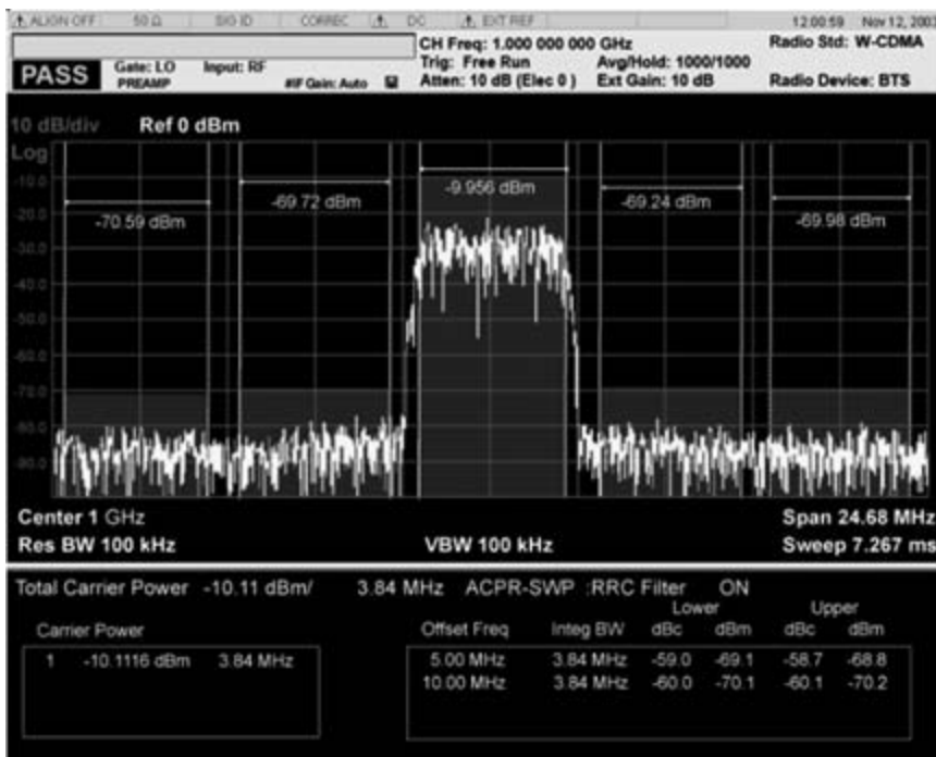
Figure 6-21 Adjacent channel power measures the impact of a signal on channels that are adjacent to it. (© Keysight Technologies, Inc. Reproduced with Permission, Courtesy of Keysight Technologies, Inc.)
