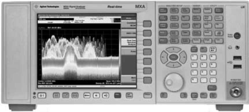
Figure 1-8 A mid-performance spectrum analyzer with a frequency range of 20 Hz to 26.5 GHz. (© Keysight Technologies, Inc. Reproduced with Permission, Courtesy of Keysight Technologies, Inc.)
