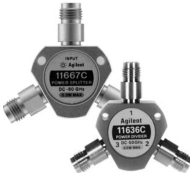
Figure 12-11 Examples of a power splitter and power divider. (© Keysight Technologies, Inc. Reproduced with Permission, Courtesy of Keysight Technologies, Inc.)
