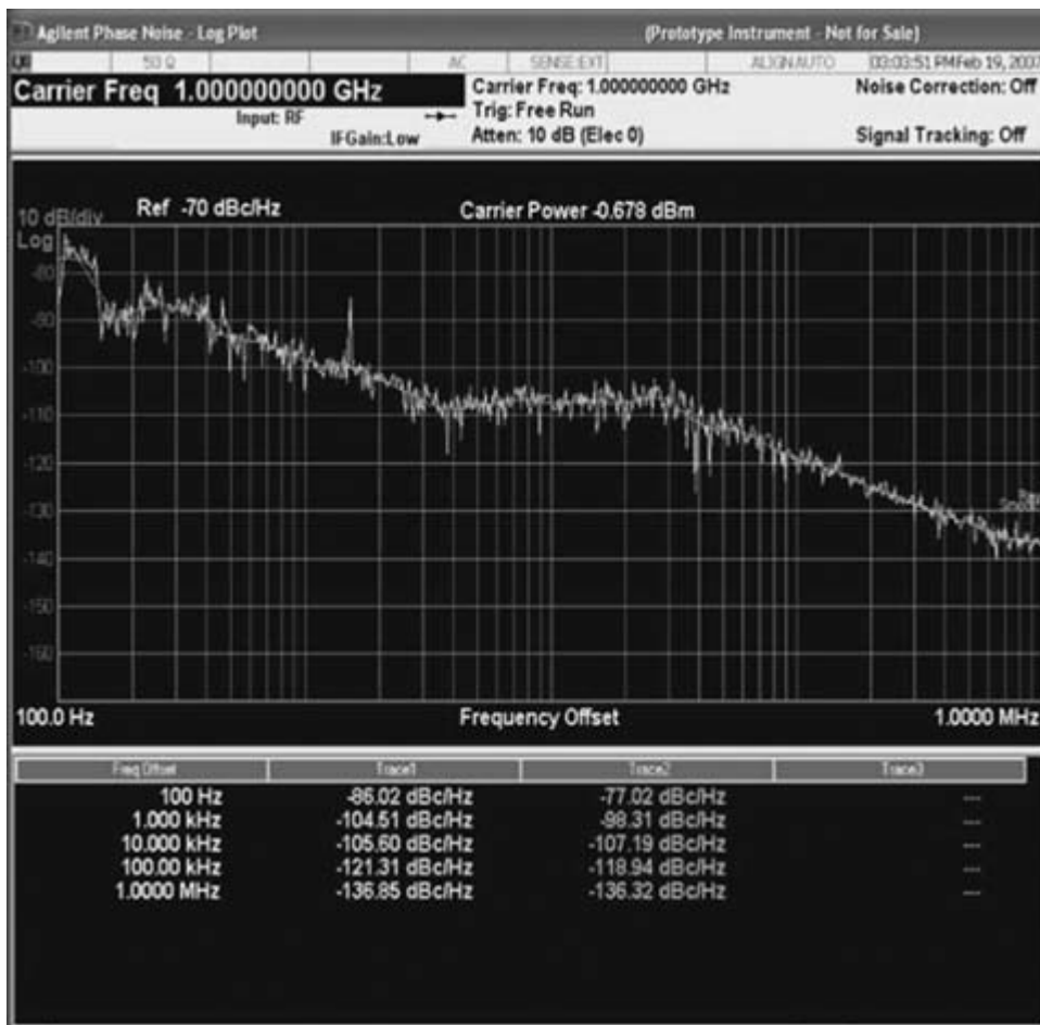
Figure 8-11 A spectrum analyzer measurement showing the single-sideband phase noise characteristics of a signal. (© Keysight Technologies, Inc. Reproduced with Permission, Courtesy of Keysight Technologies, Inc.)
