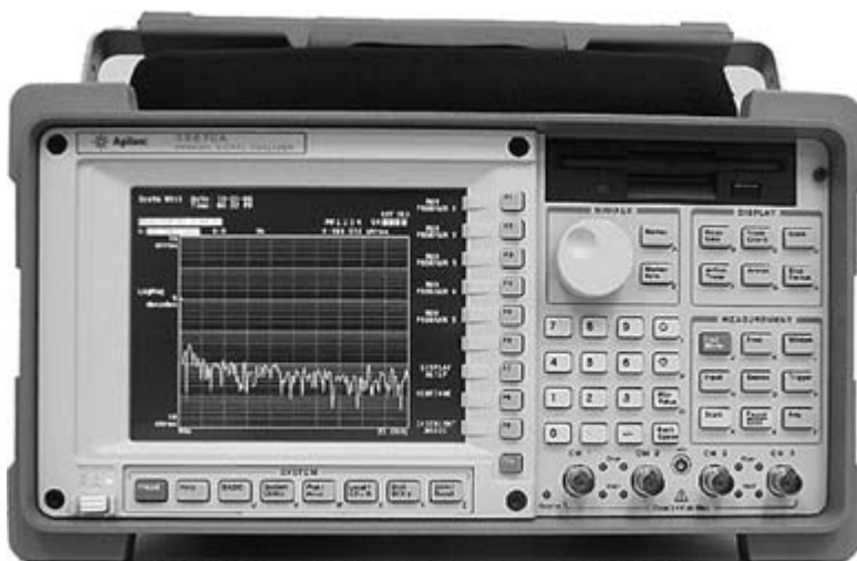
Figure 4-5 A typical four-channel FFT-based spectrum analyzer. (© Keysight Technologies, Inc. Reproduced with Permission, Courtesy of Keysight Technologies, Inc.)
