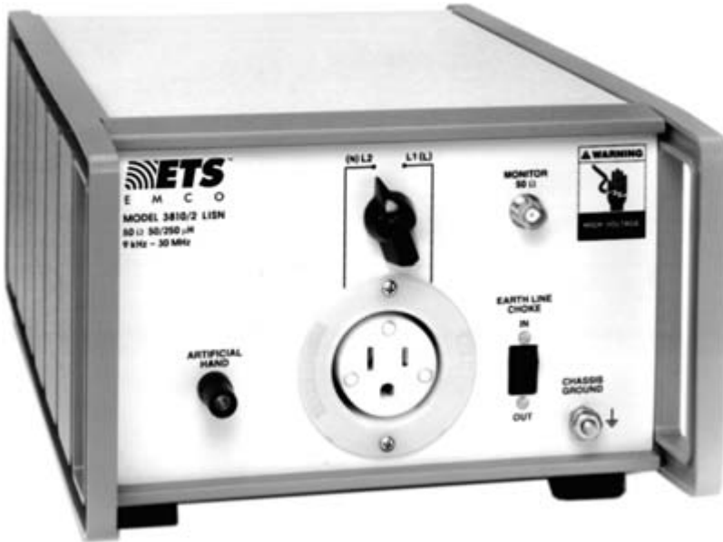
Figure 16-9 Photograph of a typical line impedance stabilization network (LISN). (Courtesy of ETS-Lindgren.)
