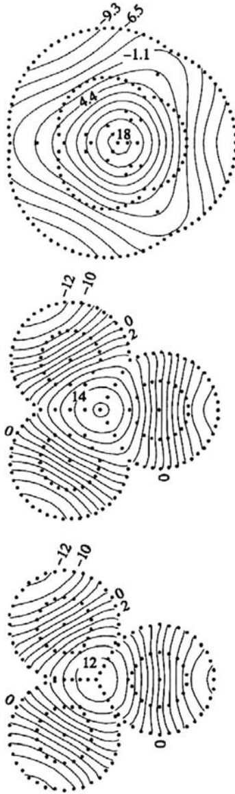
FIGURE 8.10 Equipotential lines of cloverleaf resonator with threefold symmetry, for n = 0 limit disk ( R_0/A = 0.86, 1.0, 5.0 ). (Reproduced with permission from J. Helszajn and D. J. Lynch, Cut-off space of cloverleaf resonators with electric and magnetic walls, IEEE Trans. Microwave Theory Tech. , Vol. MTT-40, No. 8, pp. 1620–1629, 1992.)
