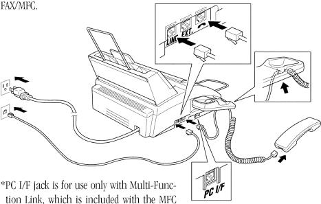
'PC I/F jack is for use only with Multi-Function Link, which is included with the MFC 1870MC and MFC 1970MC, or with the optional software. If you have not purchased the *optional* Multi-Function Link (also called "Missing Link") for your FAX 1570MC, then ignore this jack.
