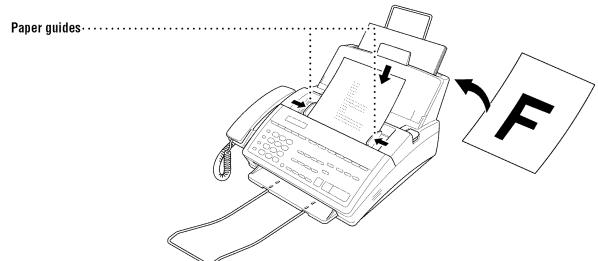
The automatic document feeder (ADF) can hold up to 20 pages, feeding each one individually through the FAX/MFC. Use standard (20 lb.) paper when using the ADF; if you're using heavier paper, feed each sheet individually to prevent paper jams.
