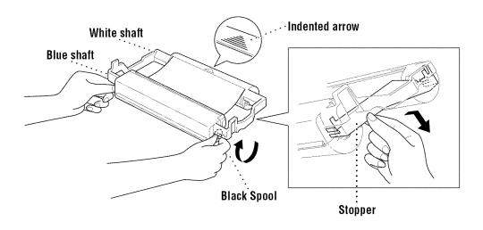
Turn the black spool on the right clockwise to tighten the ribbon, as shown.
