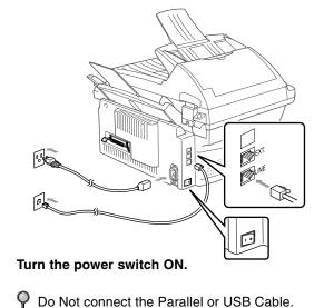
If you are sharing one phone line with an external telephone or telephone answering device (TAD), connect it as shown below.
