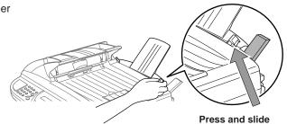
C. Push down the paper lever. Load the paper (with the lever down). Make sure the print side is toward the fax machine and the paper level is stacked below the paper mark. The feeder can hold up to 200 sheets of paper, or up to 10 envelopes.
