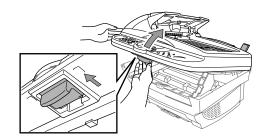
**c.** Holding the drum unit by its handles, insert it into the machine.
