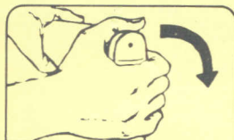
The stock butt cap is a pressure fit and removes easily.
