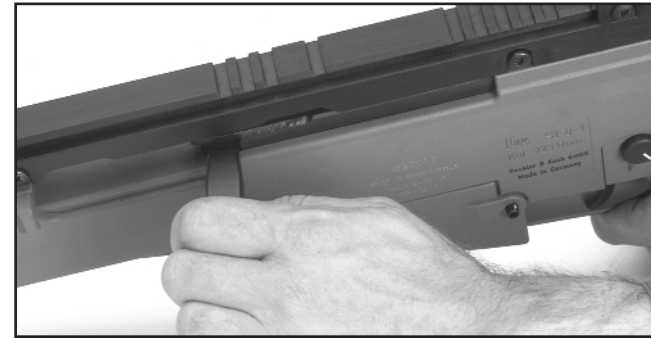
Figure 20 Operating the cocking lever
