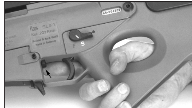
Figure 21 Activate bolt catch, push upwards
