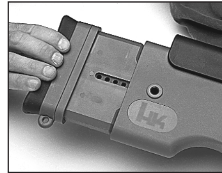
Figure 35 Remove buttplate with spacer
