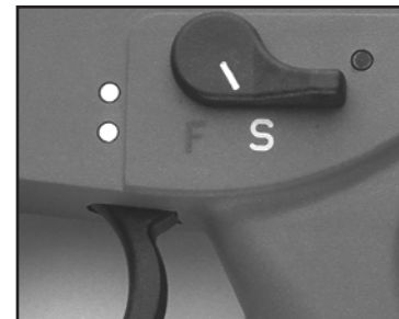
Figure 14A Safety/selector position "safe"
