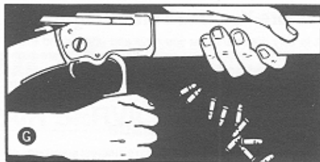
Unloading through the action
