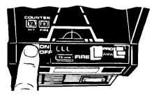
Turn the power switch off to reset the counter.
