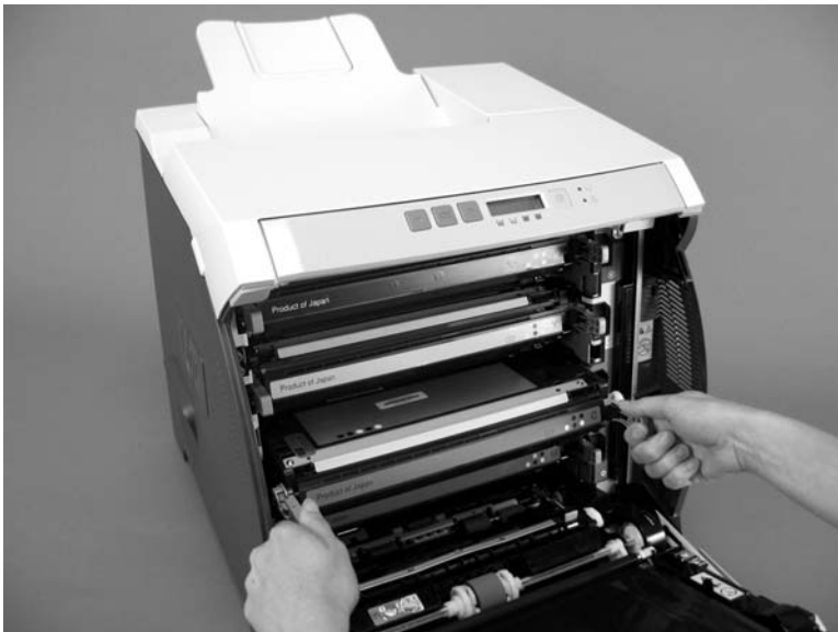
Figure 5-3 Remove the print cartridges (2 of 2)
