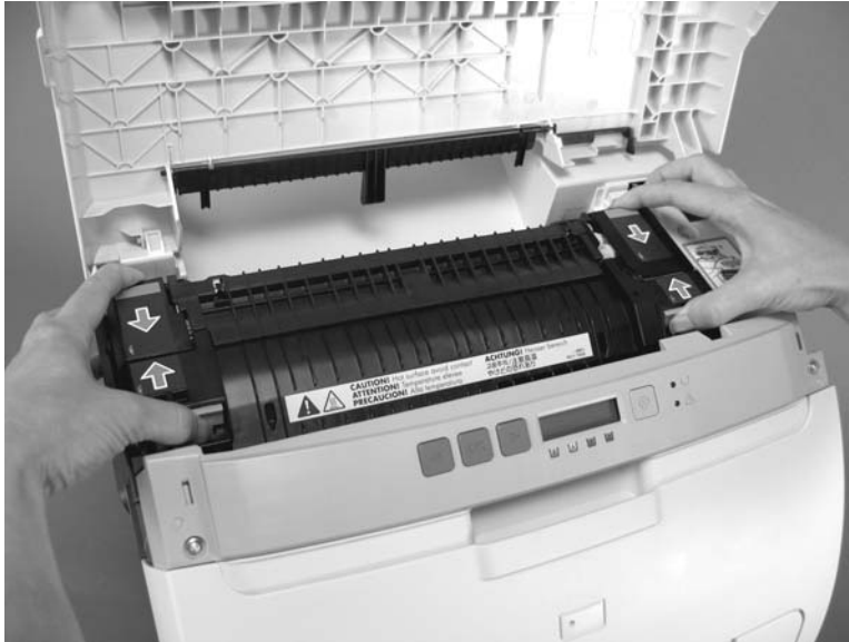
Figure 5-28 Remove the fuser
