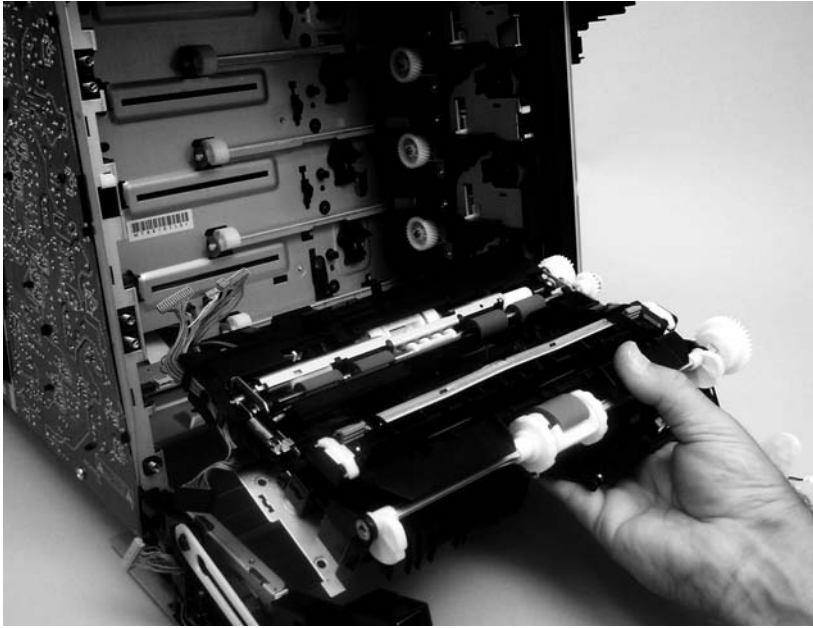
Figure 5-47 Remove the pickup-and-feed assembly (8 of 8)
