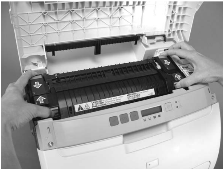
Figure 5-10 Remove the upper cover (2 of 5)
