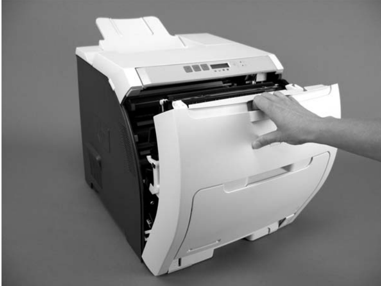
Figure 5-2 Remove the print cartridges (1 of 2)
