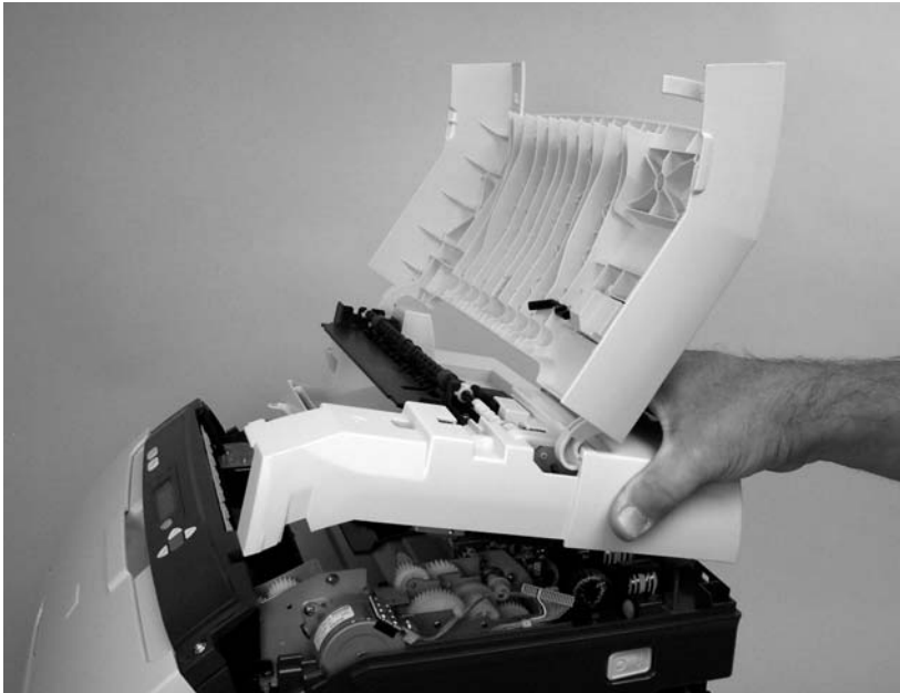
Figure 5-13 Remove the upper cover (5 of 5)
