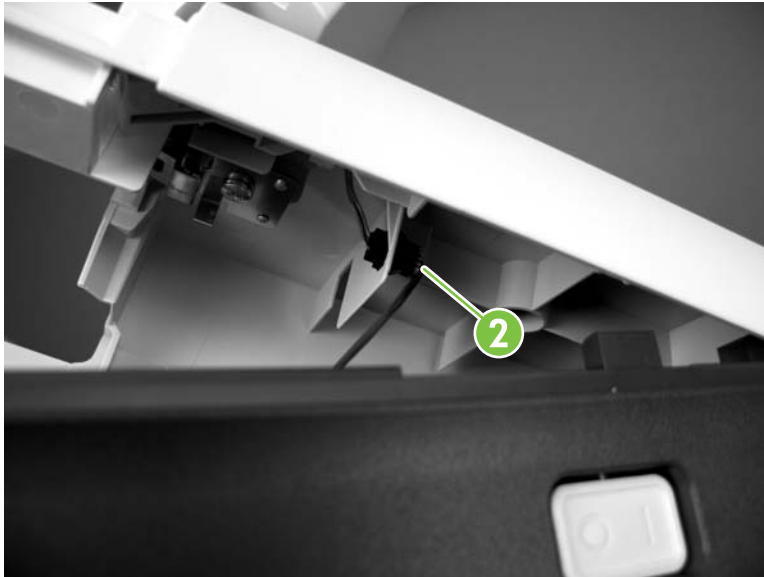
Figure 5-12 Remove the upper cover (4 of 5)
