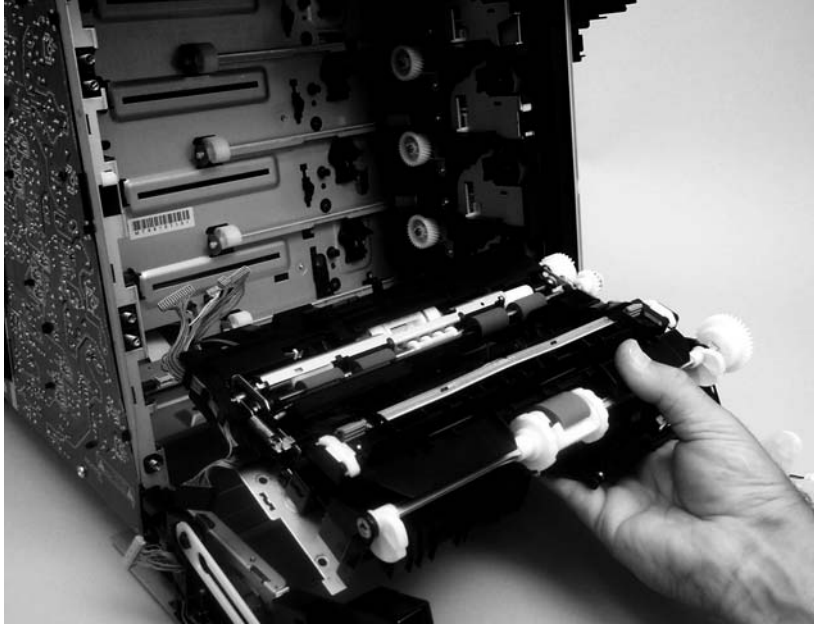
Figure 5-57 Remove the pickup-and-feed assembly (8 of 8)
