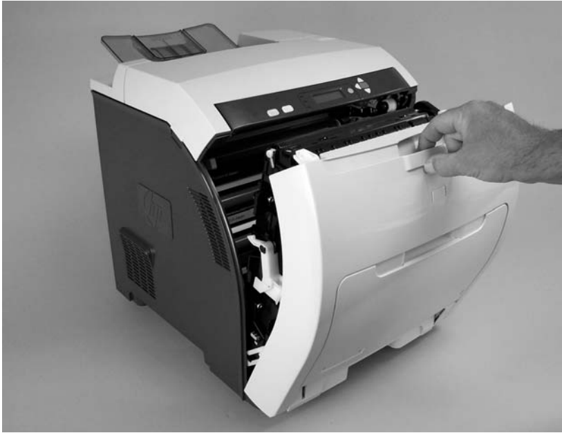
Figure 5-2 Remove the print cartridges (1 of 2)
