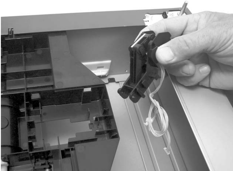
Figure 5-127 Remove the media sensor (500-sheet feeder) (4 of 4)
