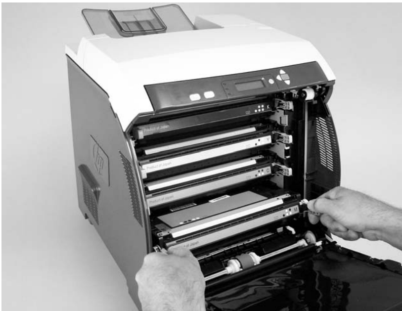
Figure 5-3 Remove the print cartridges (2 of 2)
