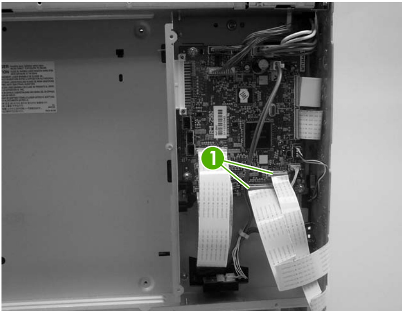
Figure 5-88 Remove the high-voltage power supply (1 of 3)
