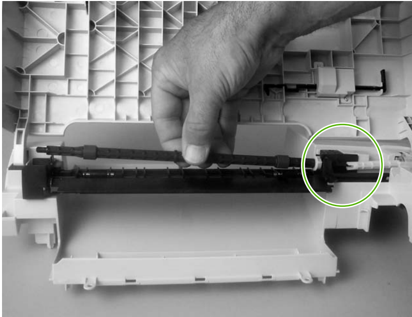
Figure 5-36 Remove the duplex-reverse-drive assembly (2 of 5)
