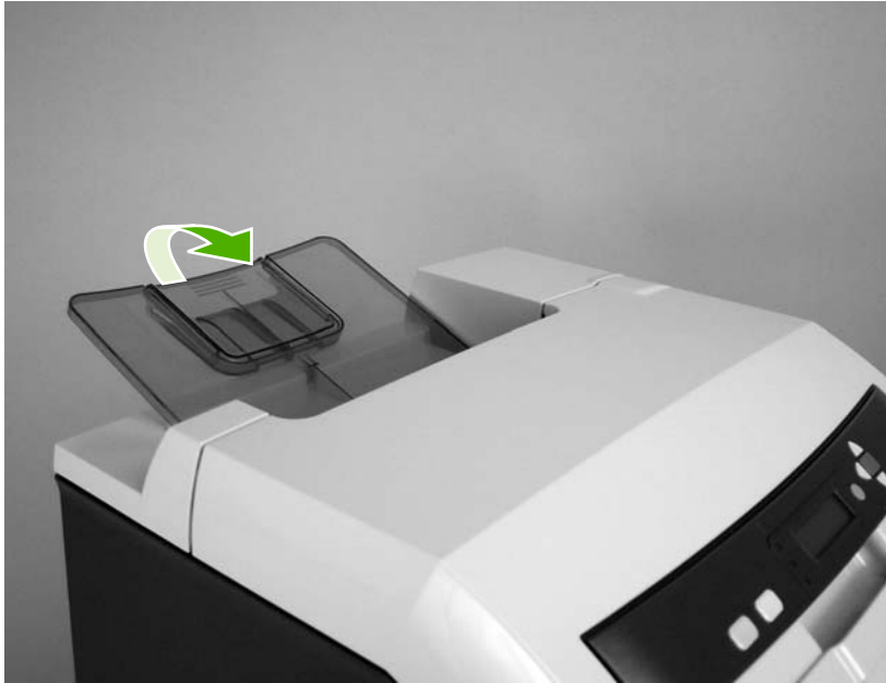
Figure 5-11 Remove the upper cover (1 of 5)
