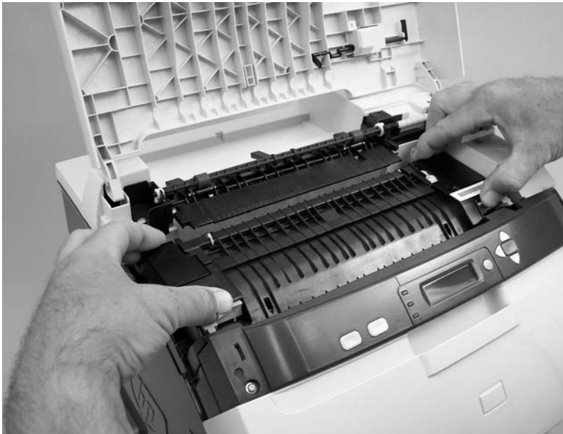
Figure 5-12 Remove the upper cover (2 of 5)
