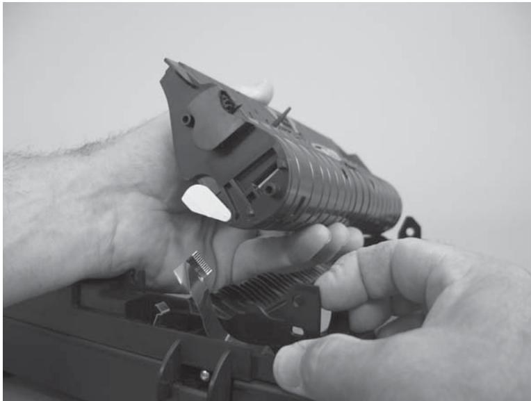
Figure 1-100 Remove the document feeder core (4 of 4)
