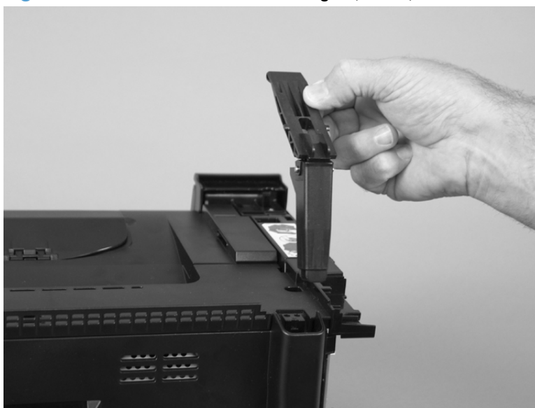
Figure 1-18 Remove the scanner hinges (2 of 2)
