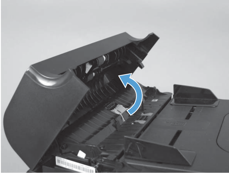
Figure 1-94 Remove the document feeder cover (1 of 3)
