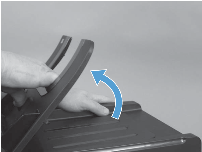
Figure 1-93 Remove the document feeder input tray (2 of 2)
