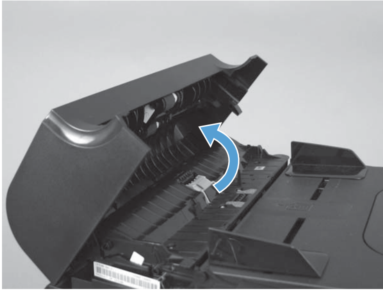
Figure 1-92 Remove the document feeder input tray (1 of 2)
