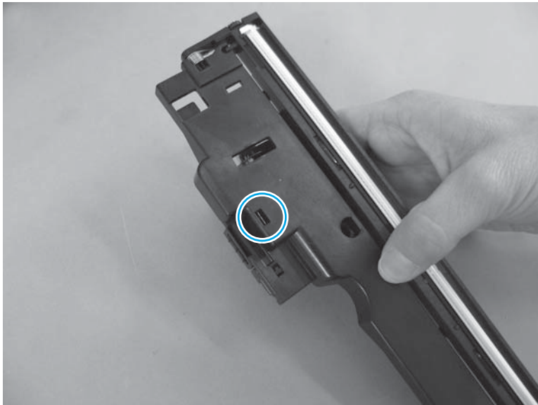
Figure 1-126 Reinstall the scan motor
