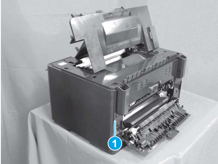
Figure 1-17 Remove the right cover (1 of 3)
