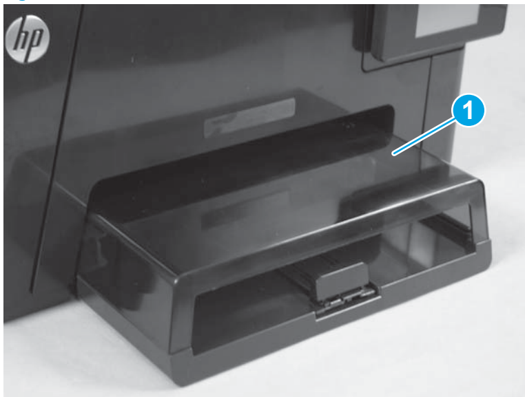
Figure 1-3 Remove the dust cover
