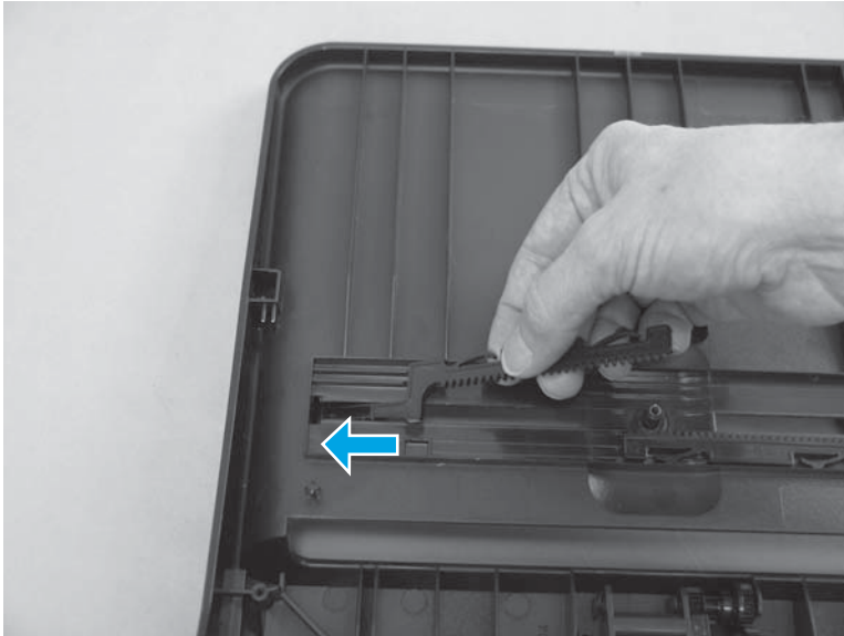
Figure 1-144 Remove the ADF input guides and gear (2 of 3)
