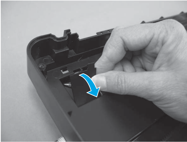
Figure 1-122 Remove the scan FFC cable (2 of 3)
