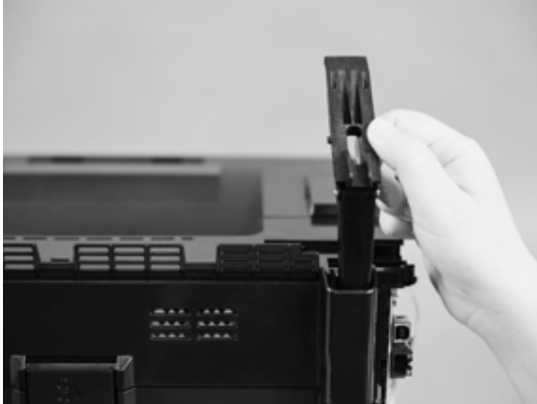
Figure 1-21 Remove the scanner hinges (2 of 2)
