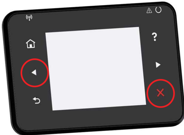
Figure 2-1 Control-panel 2ndary Service test access buttons
