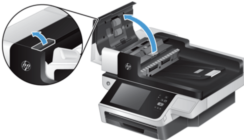
Figure 2-1 Remove the ADF rollers (1 of 1)
