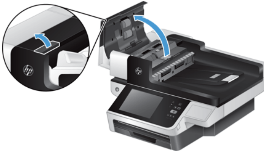
Figure 2-5 Remove the separation pad (1 of 3)
