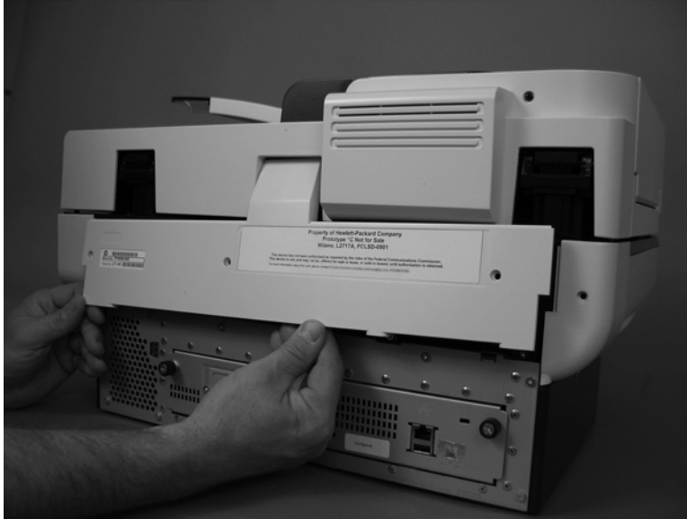
Figure 2-34 Remove the flatbed scanner and ADF assembly (4 of 7)
