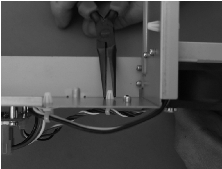
Figure 2-62 Remove the fan assembly (1 of 3)
