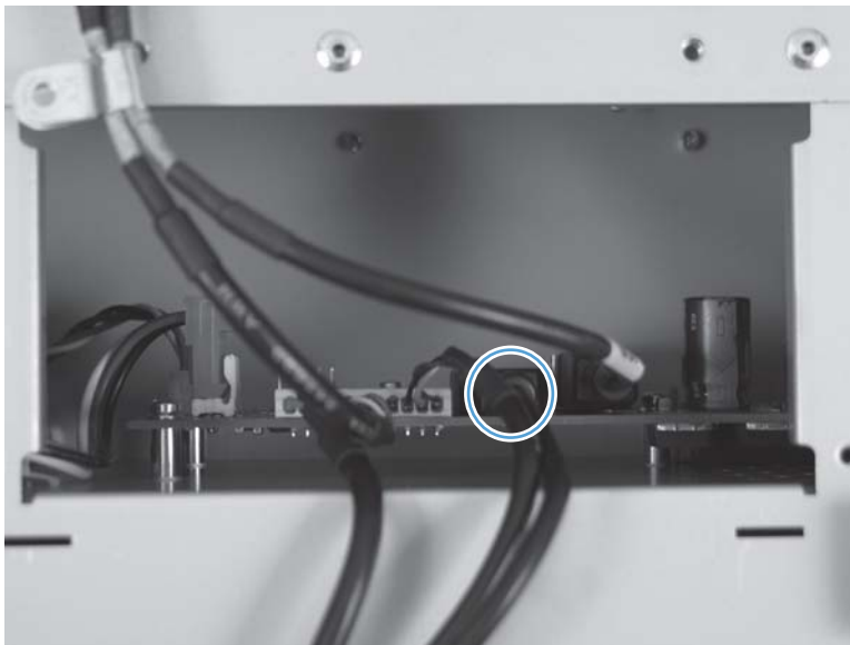
Figure 2-48 Remove the control-panel cable (1 of 3)
