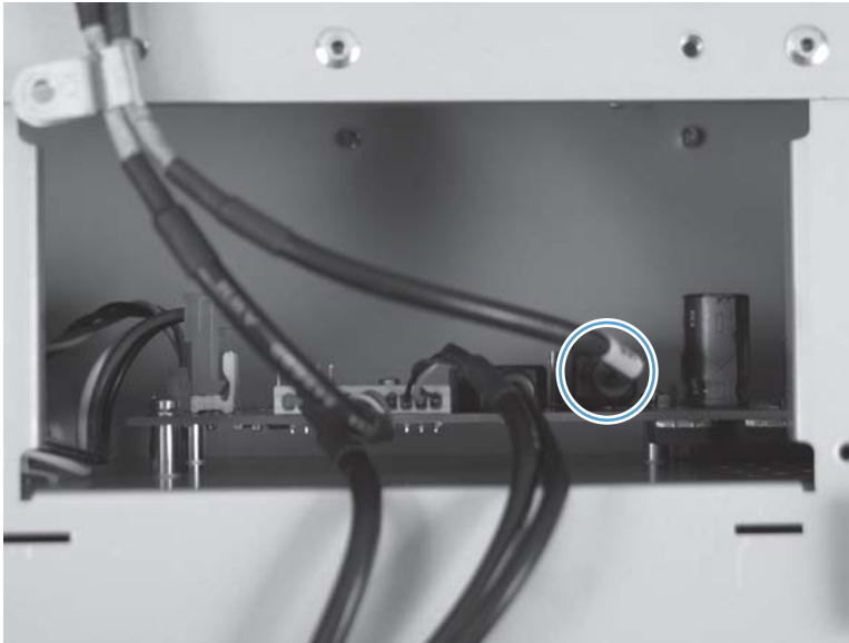
Figure 2-45 Remove the scanner cable (1 of 3)
