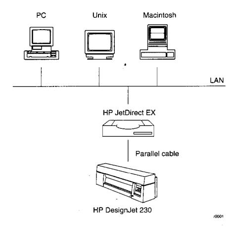
For installation of the HP JetDirect EX interface, see the Installation Guide that comes with that product.
