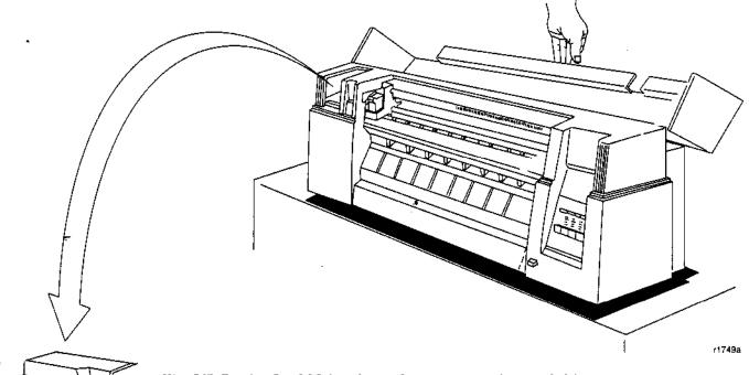
The HP DesignJet 230 is a large format monochrome inkjet plotter. It uses a **single disposable print cartridge**, which is held in an easy-to-access cartridge carriage.
