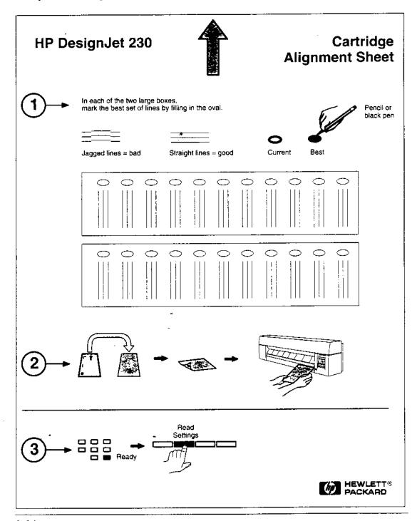
When the plot has finished, wait until the **Load Media** light comes on and the plotter ejects the sheet – plus one and a half minutes for the ink to dry – and then remove it. Follow the instructions on the sheet itself. As you will see, this involves you identifying the straightest set of vertical lines in each of the two boxes.
