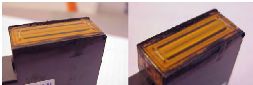
Ink accumulation at the bottom edges of the Printheads.
