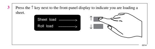
Press the  $\uparrow$  or  $\downarrow$  key until the display shows the type of media you are loading (if you are using heavyweight coated paper, scroll to Heavy coated paper), and then press the **Enter** key.
