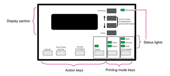
The front panel of the HP DesignJet 755CM printer is shown below:
