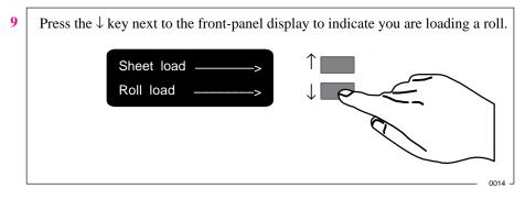
Press the  $\uparrow$  or  $\downarrow$  key until the display shows the type of media you are loading (for example, if you are using the roll of HP Heavyweight Coated Paper supplied with the printer, scroll to Heavy coated paper) and then press the **Enter** key.
