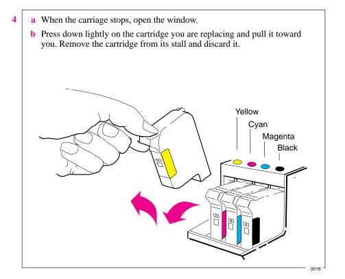
5 Notice that each stall in the carriage has a dot indicating the color: when loading the new cartridge you *must* put the correct cartridge in the correct stall.
