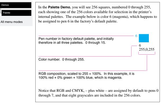
The 256 colors shown in the Palette Demo are not the only colors you can print with your printer! Using your software, you can create many more colors and, as long as you are using the correct driver, the printer will reproduce these colors by an appropriate mix of inks from its CMYK cartridges. The Palette Demo merely shows the 256 colors available for use in the printer's internal palettes, should you choose to use them.
