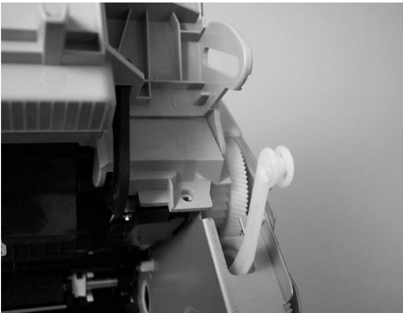
Figure 5-12 Remove the rear panel and top-cover assembly (3 of 6)
