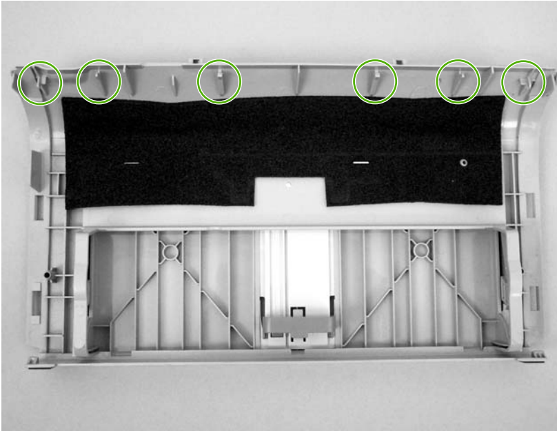
Figure 5-18 Remove the front cover (1 of 3)
