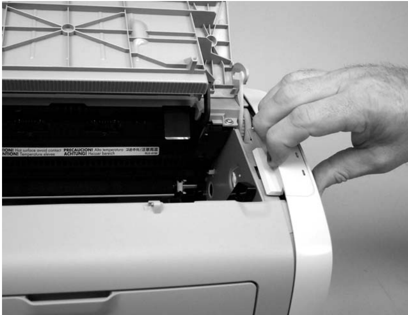
Figure 5-8 Remove the right-side cover (3 of 4; HP LJ 1020 printer shown)
