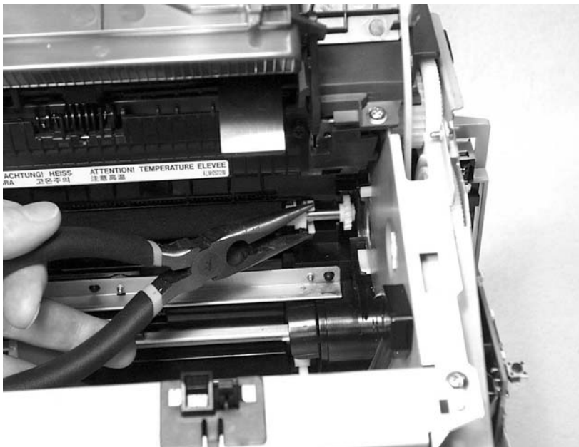
Figure 5-23 Remove the transfer roller (3 of 3)
