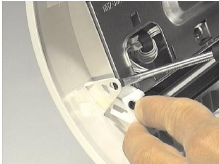
Figure 4-5 Removing the Contact Image Sensor (continued)
