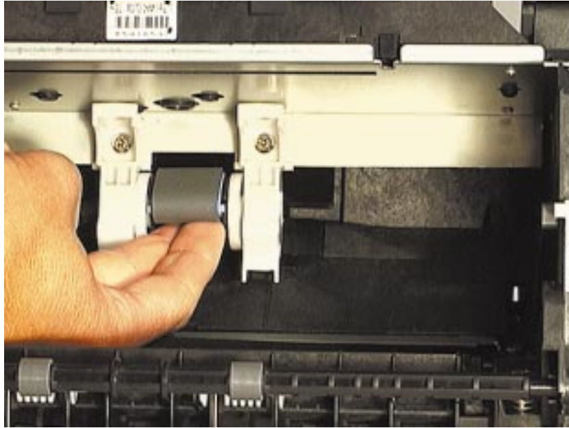
Figure 4-38 Changing the pickup roller
