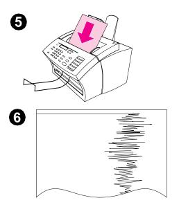
The HP LaserJet 3100 product was calibrated at the factory. However, you may need to recalibrate the scanner if you notice that sent faxes, copies, or items scanned to the computer have black or white lines running through them.
