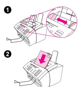
Whether you want to fax, copy, or scan, the procedure for loading the document is the same. If your document is on a regular weight paper (from 12 to 28 lb or 46 to 105 g/m²), use "To load normal items." If your document is a transparency, in a carrier sheet, or is not on regular weight paper, use "To load special items."
