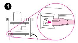
The HP LaserJet 3100 product does not have a power switch. It turns on when the power cord is connected.
