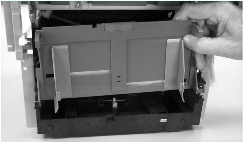
Figure 78. Removing the paper lift-plate assembly (3 of 3)
