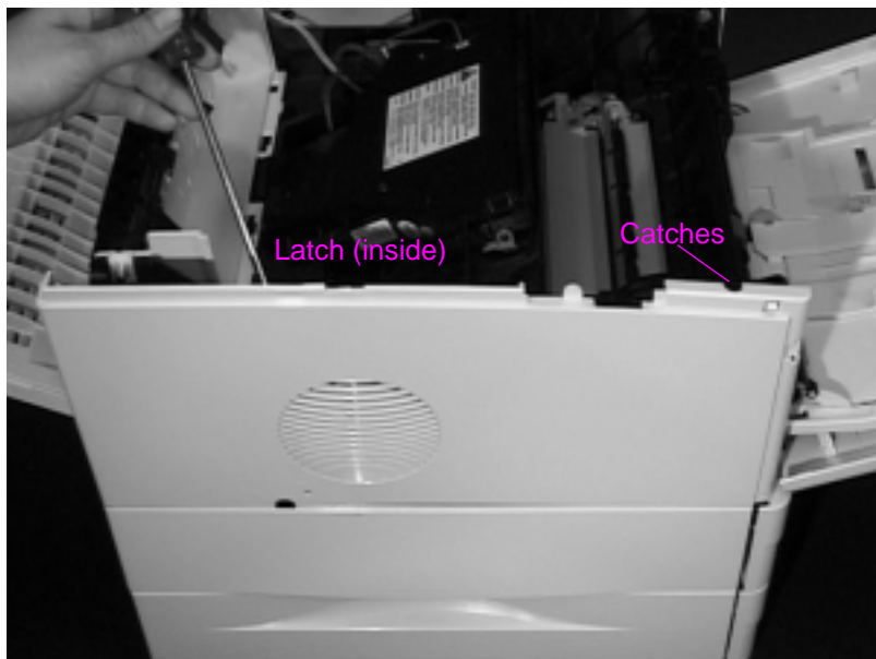
Figure 6-8 Removing the Left Side Cover
