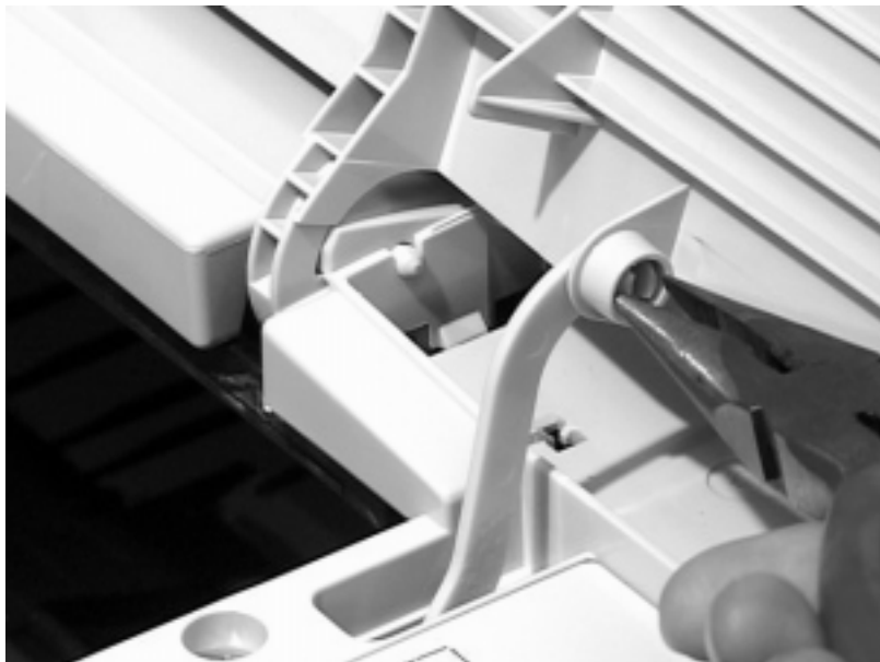
Figure 6-5 Removing the Toner Cartridge Drive Arm
