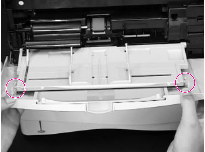
Figure 6-11 Removing Tray 1 from the Front Cover
