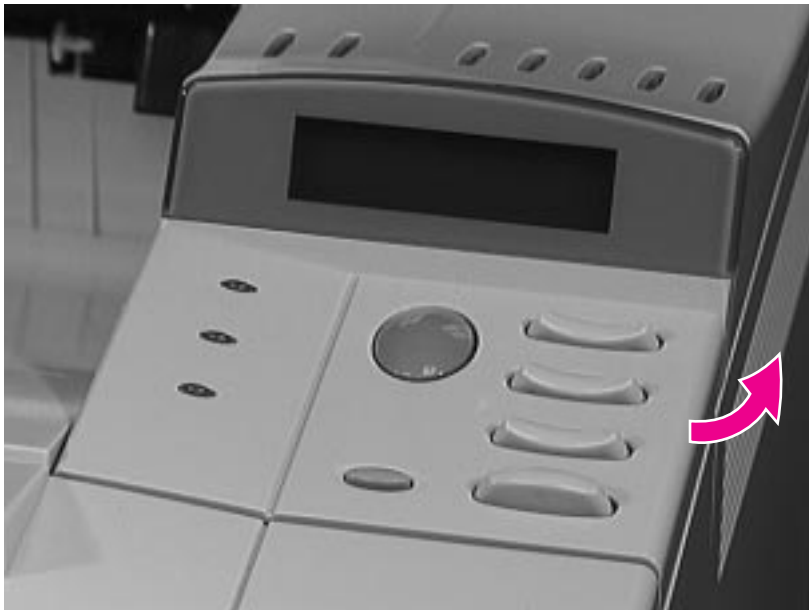
Figure 6-3 Removing the Control Panel Overlay
