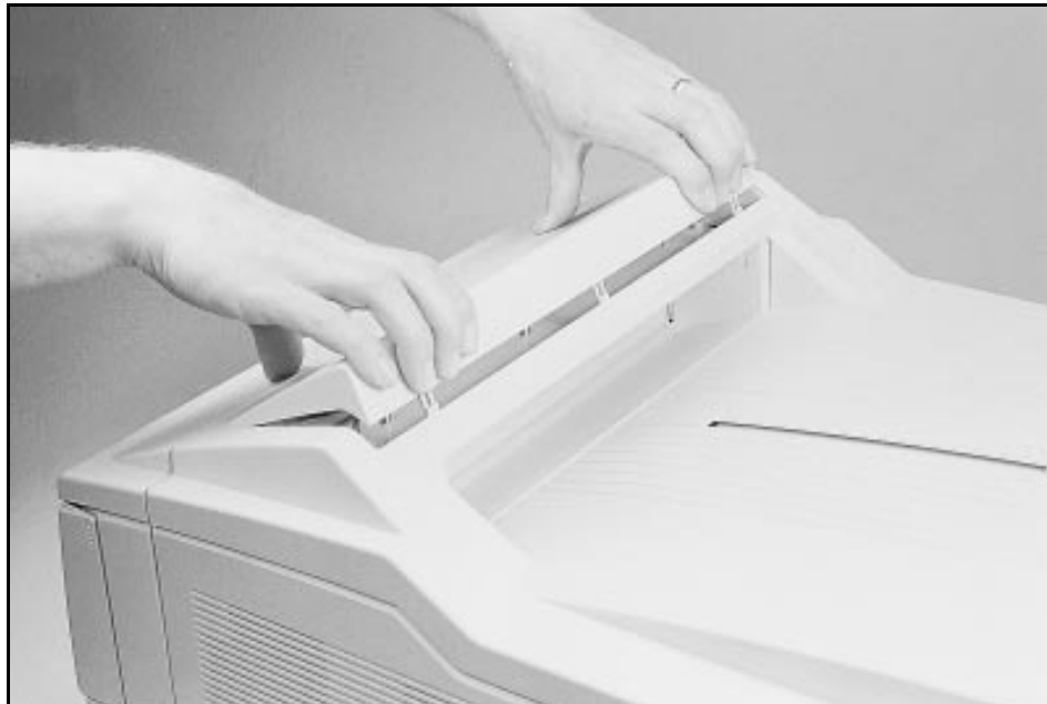
Removing the Control Panel
