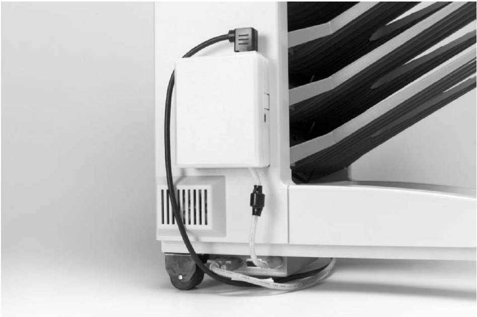
Figure 7-24 8-bin Mailbox Power Supply Test Mode Switch
