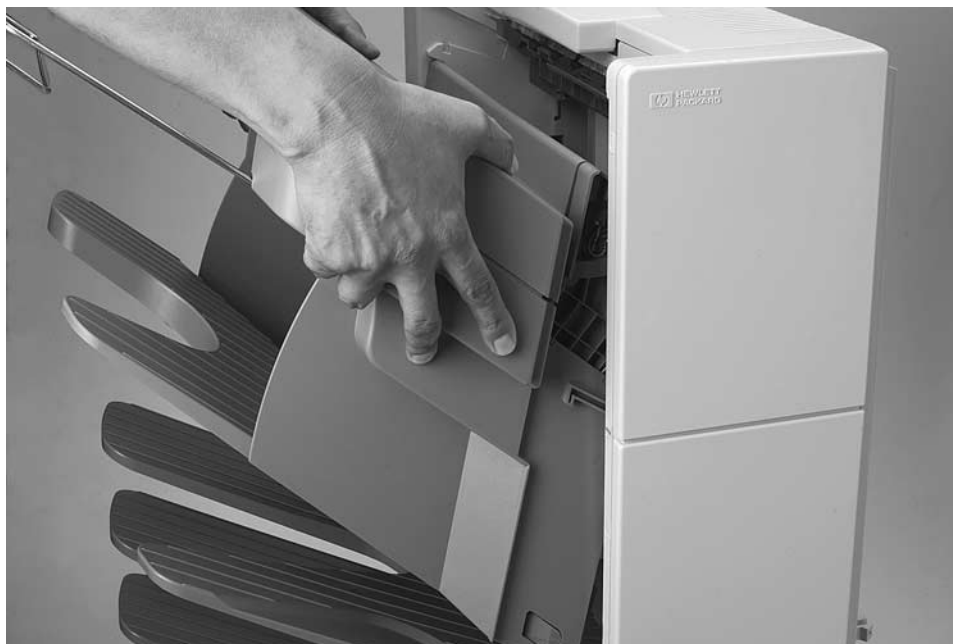
Figure 6-180 Mailbox with Stapler, Stapler Removal or Installation
