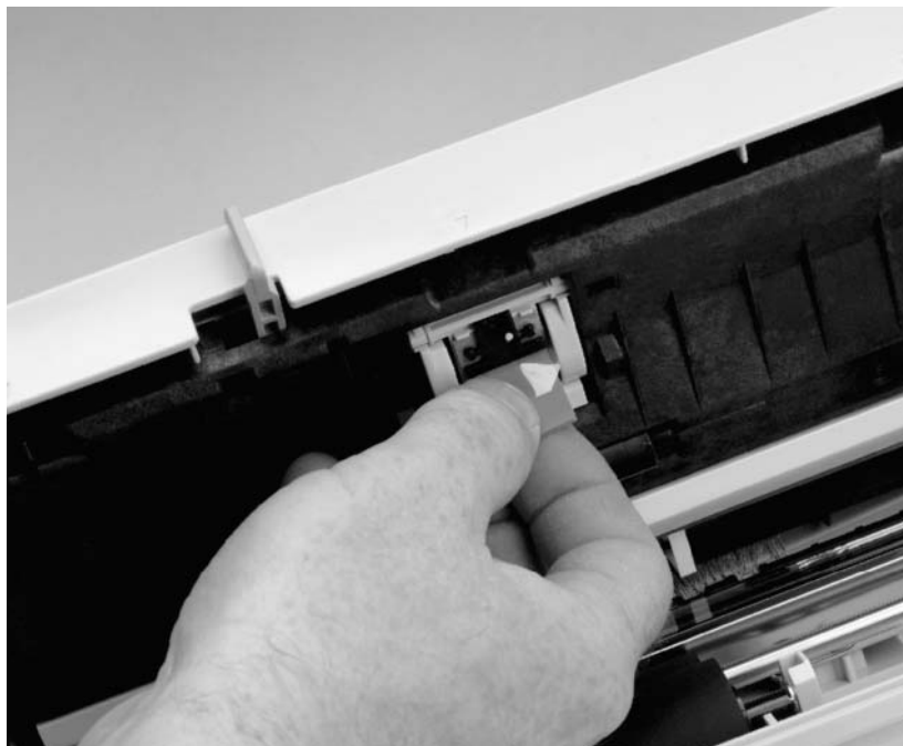
Figure 34. Document scanner separation pad removal
