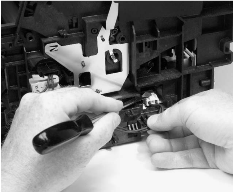
Figure 50. Fusing element removal (3 of 4)
