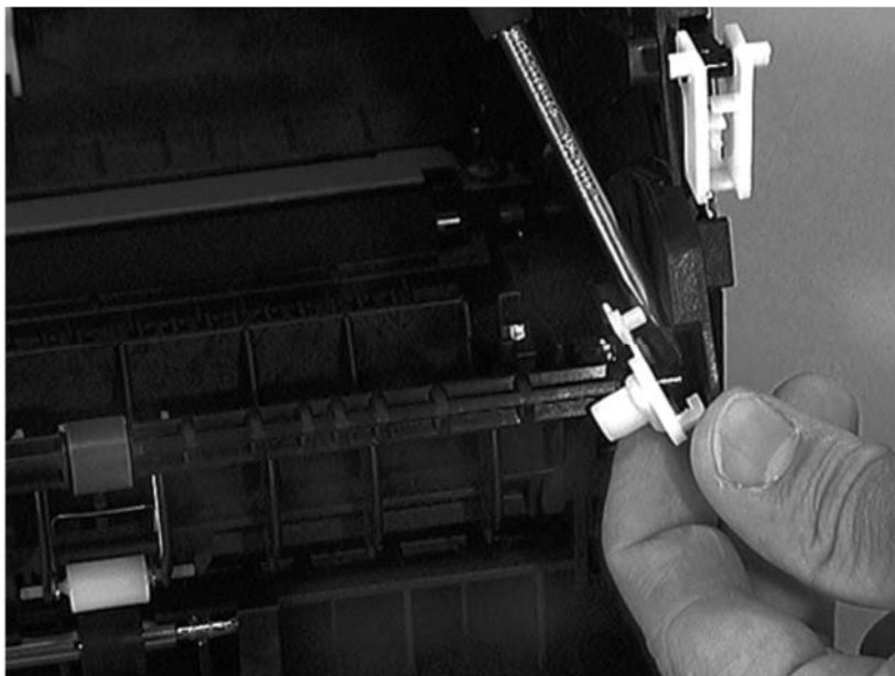
Figure 42. Output roller removal (1 of 2)
