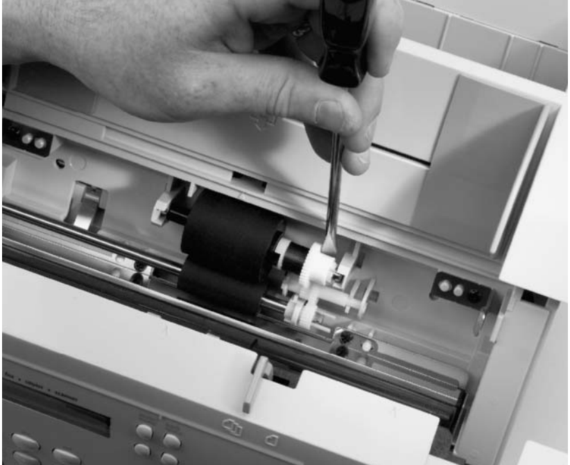
Figure 33. Document scanner pickup roller removal
