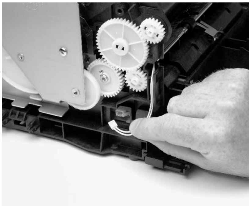
Figure 49. Fusing element removal (2 of 4)
