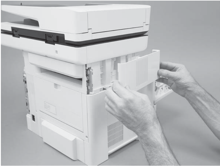
Figure 1-1917 Remove the cover
