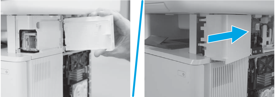
Figure 1-770 Install the door or cover
