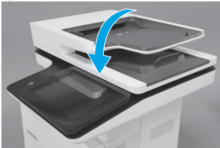
Figure 1-792 Close the document feeder
