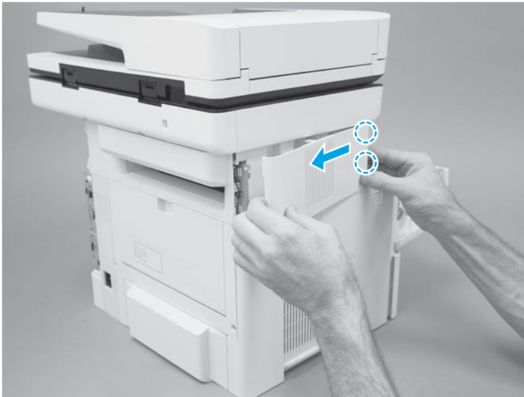
Figure 1-178 Slide the cover
