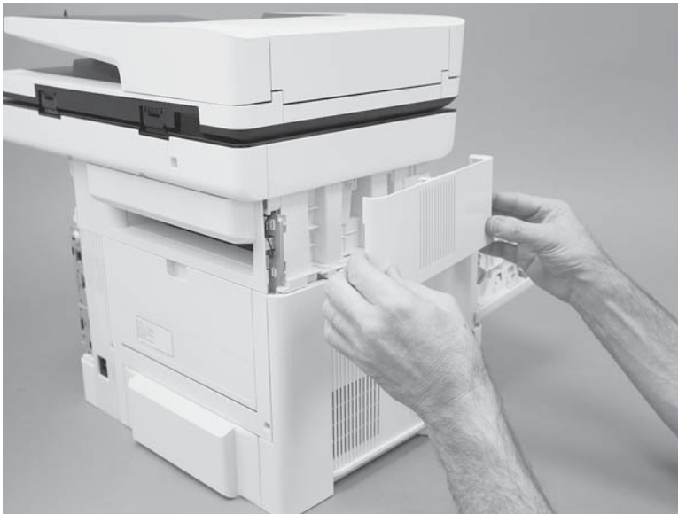
Figure 1-204 Remove the cover
