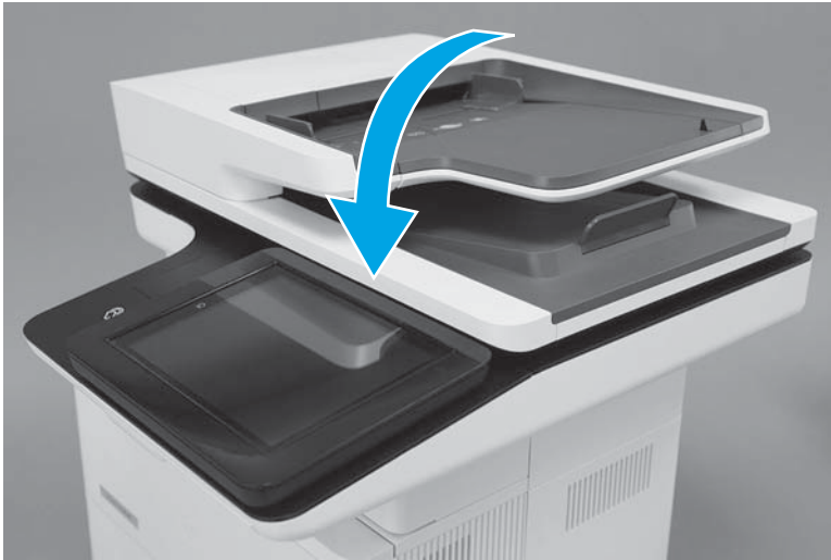
Figure 1-91 Close the document feeder
