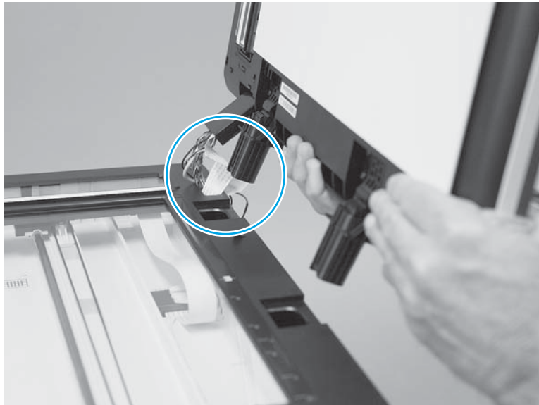
Figure 1-214 Remove the document feeder
