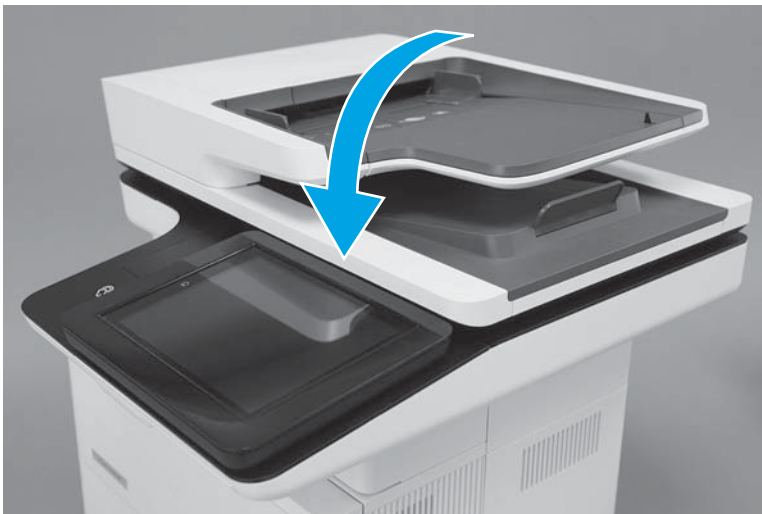
Figure 1-69 Close the document feeder
