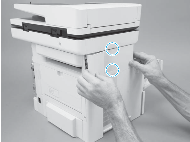
Figure 1-875 Engage two tabs
