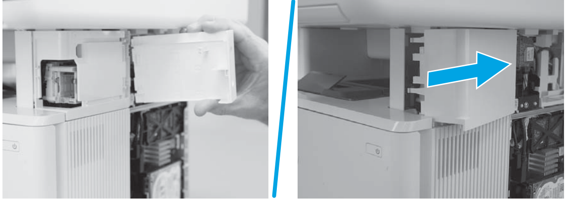
Figure 1-973 Install the door or cover
