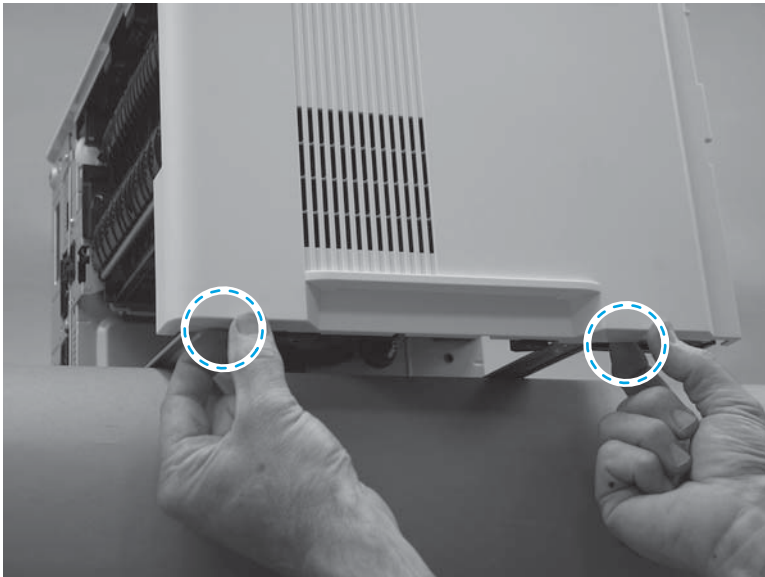
Figure 1-321 Engage two tabs
