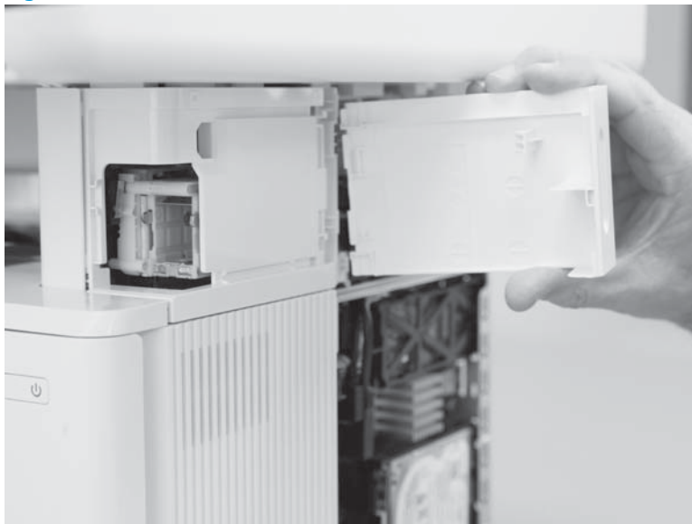
Figure 1-1022 Remove the door
