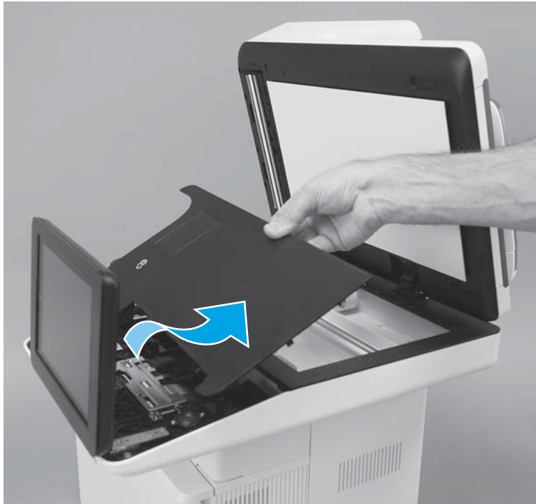
Figure 1-696 Remove the cover
