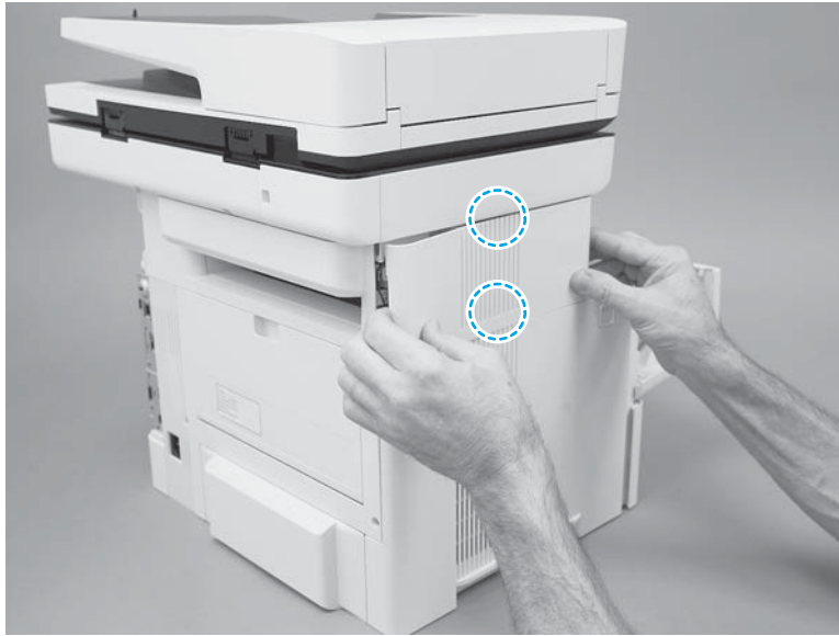
Figure 1-764 Engage two tabs
