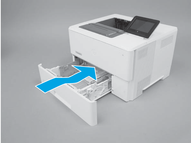
Figure 1-1675 Install the tray
