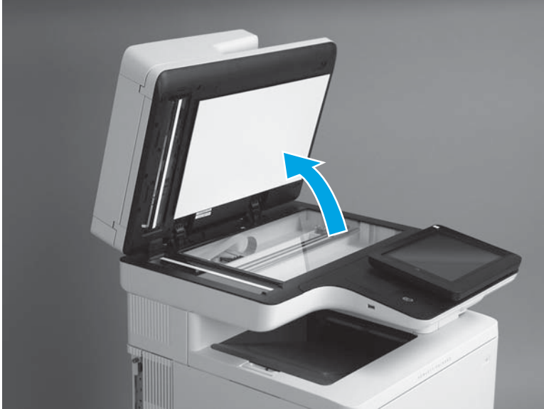
Figure 1-92 Open the document feeder
