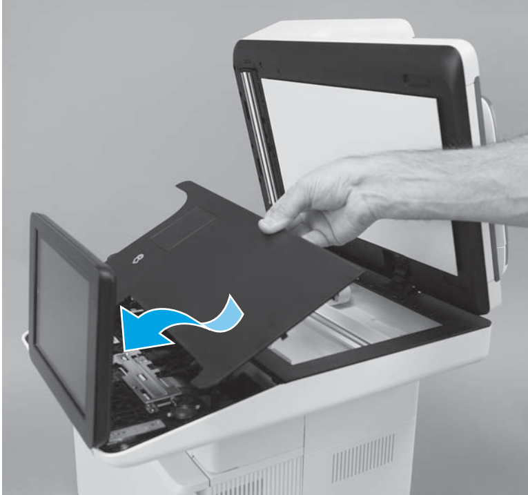
Figure 1-886 Position the control-panel cover on the printer
