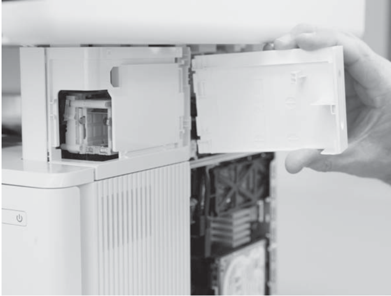
Figure 1-1909 Remove the door
