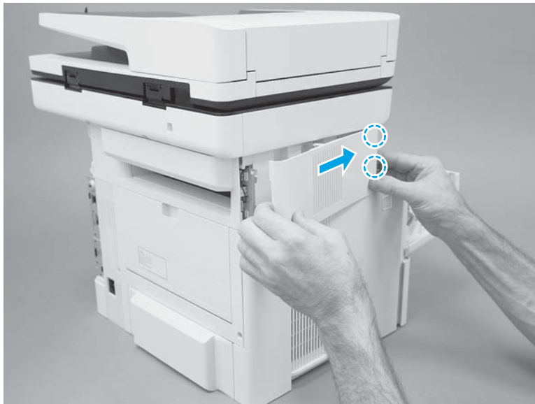
Figure 1-230 Slide the cover
