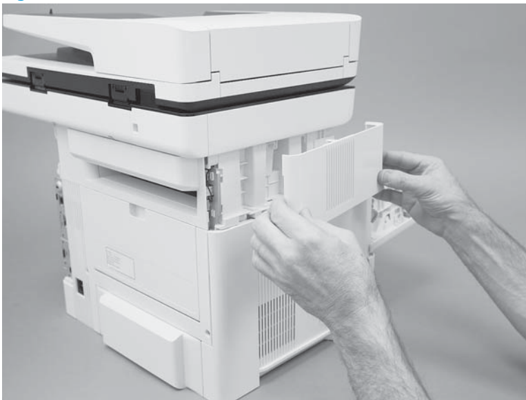
Figure 1-195 Remove the cover
