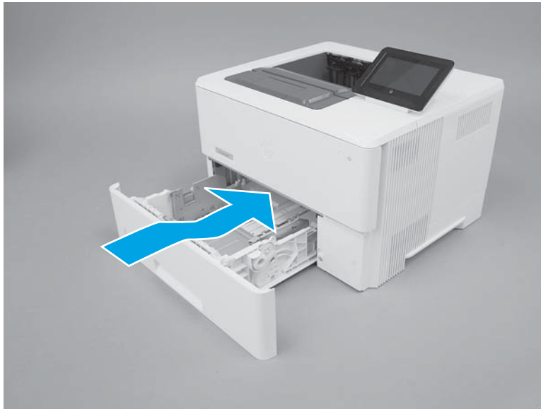
Figure 1-148 Install the tray
