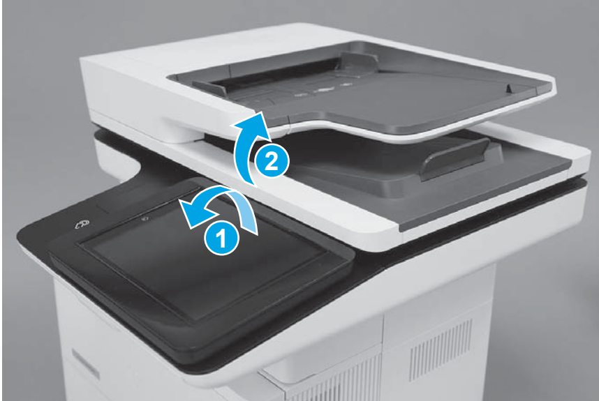
Figure 1-50 Open the document feeder
