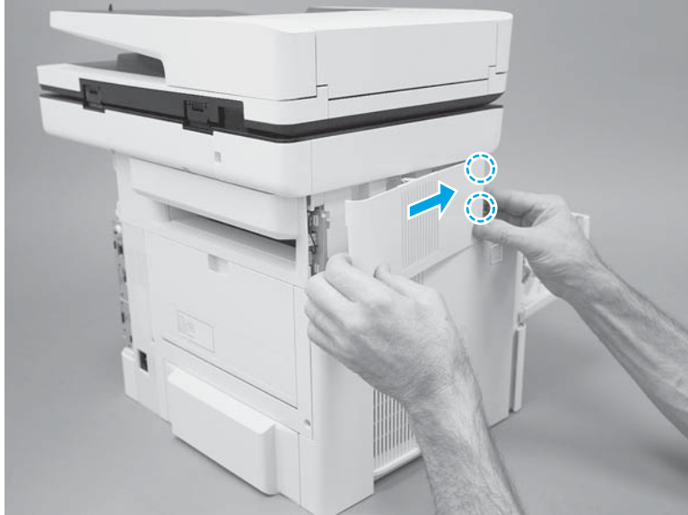
Figure 1-874 Slide the cover
