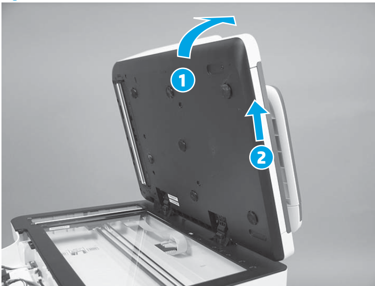
Figure 1-731 Raise the document feeder
