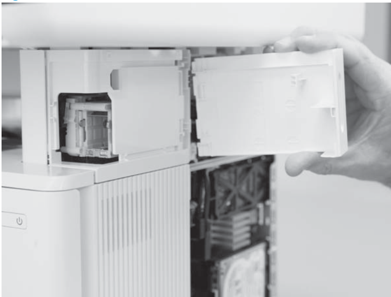
Figure 1-374 Remove the door
