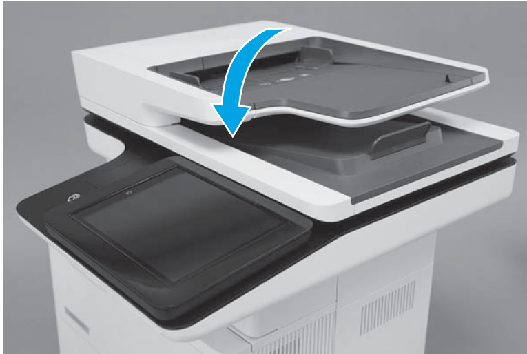
Figure 1-888 Close the document feeder
