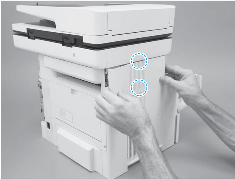
Figure 1-189 Engage two tabs
