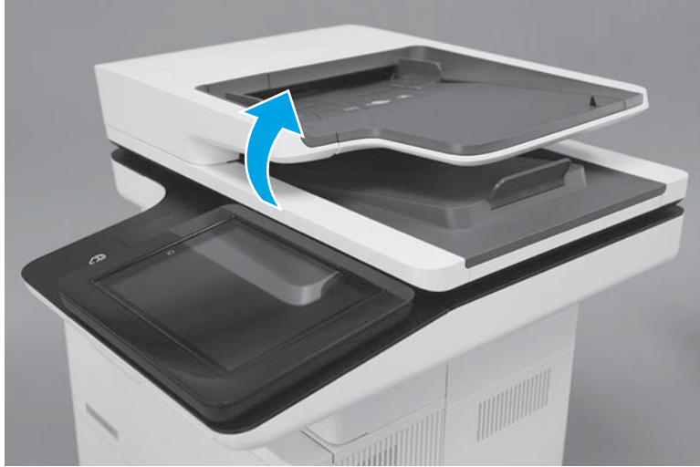
Figure 1-81 Open the document feeder
