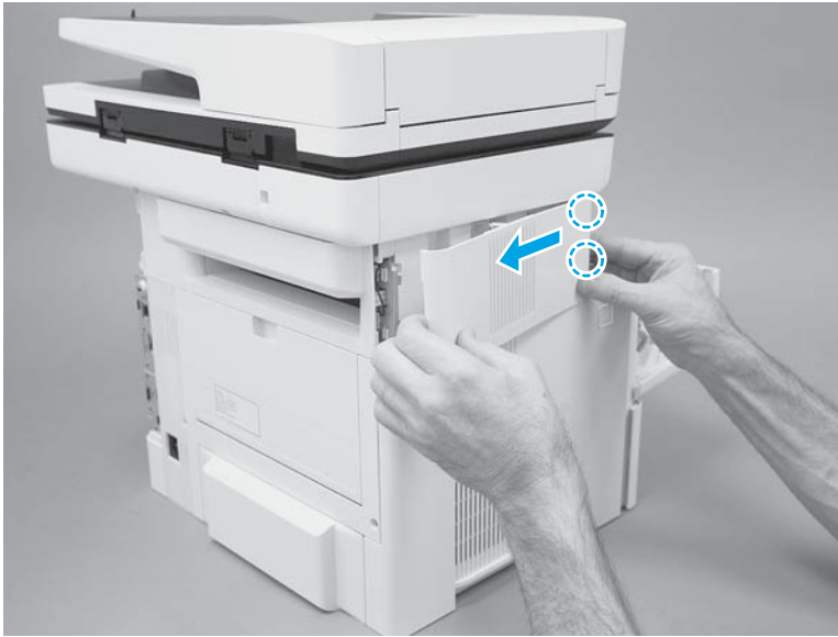
Figure 1-381 Slide the cover
