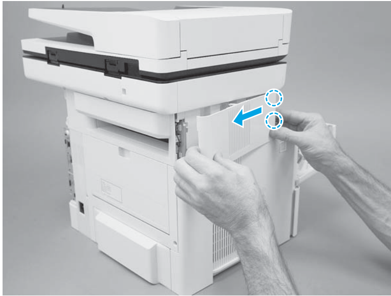
Figure 1-1029 Slide the cover
