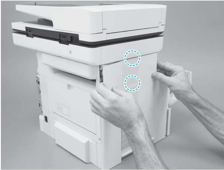
Figure 1-231 Engage two tabs
