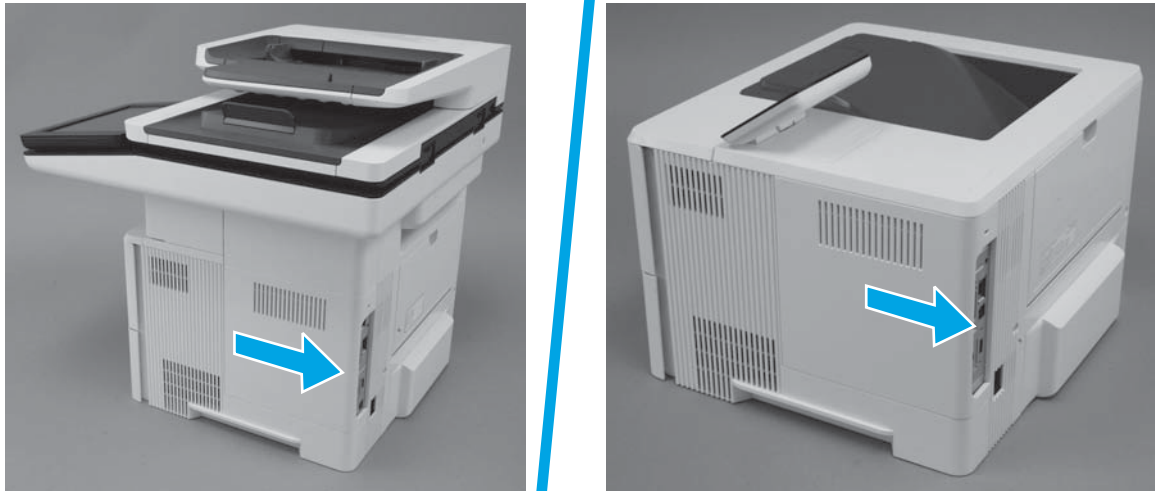
Figure 1-843 Remove the formatter cover
