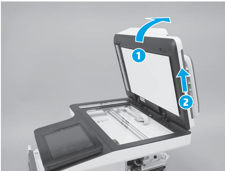
Figure 1-212 Raise the document feeder
