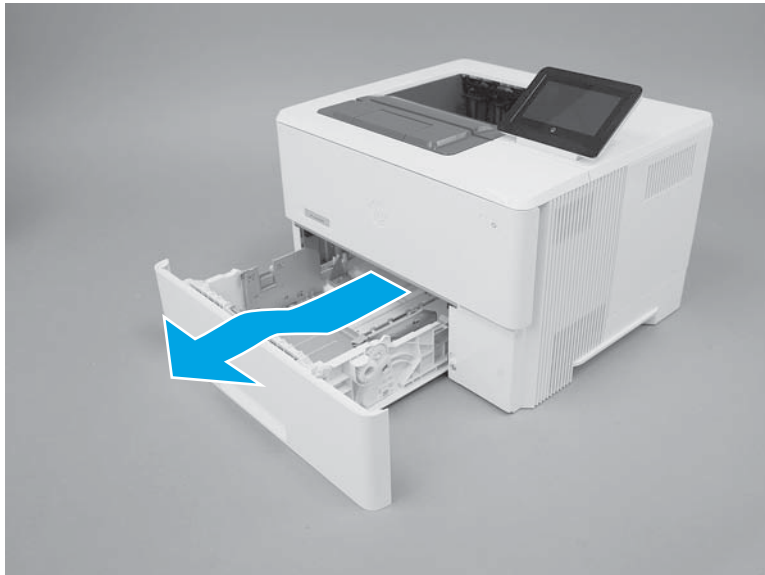
Figure 1-1355 Release and remove the tray
