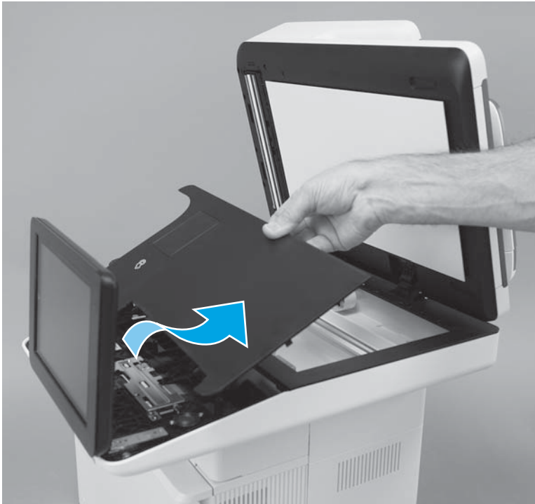
Figure 1-106 Remove the cover
