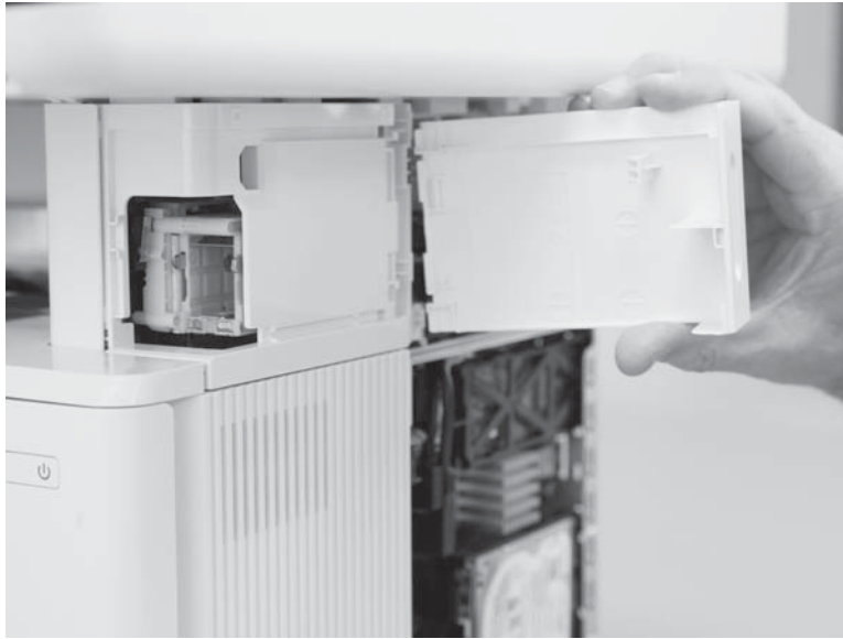
Figure 1-1166 Remove the door
