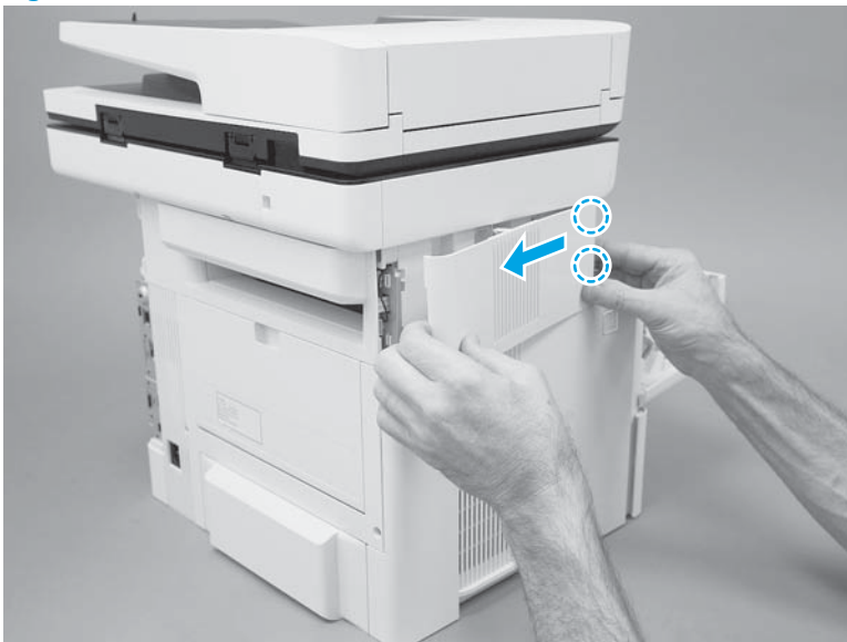
Figure 1-1540 Slide the cover
