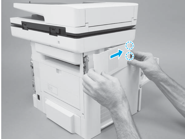
Figure 1-1278 Slide the cover
