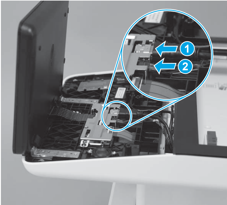
Figure 1-64 Connect the connectors
