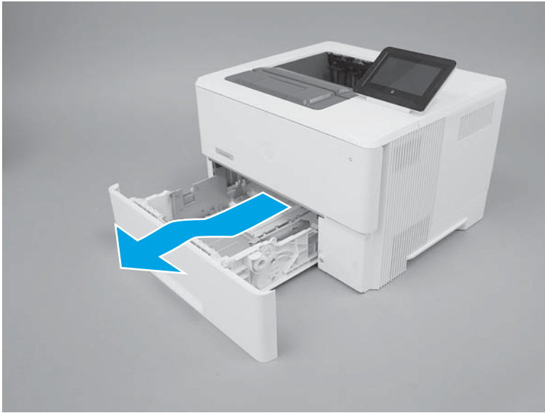
Figure 1-134 Release and remove the tray
