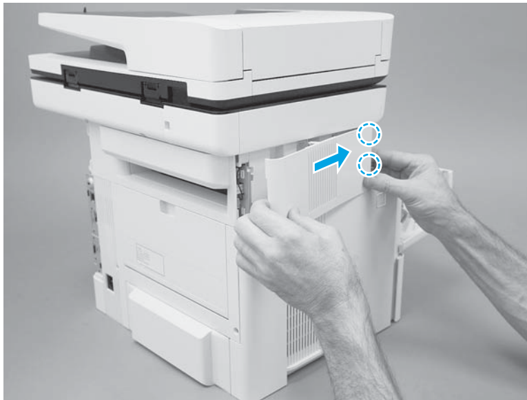
Figure 1-188 Slide the cover
