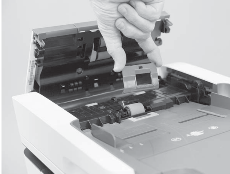
Figure 1-2089 Remove the cover
