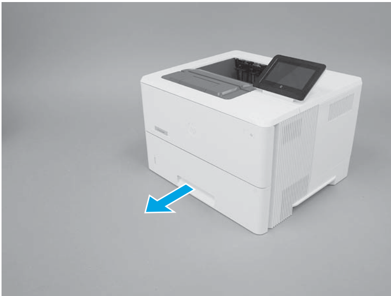
Figure 1-1846 Pull the tray out until it stops
