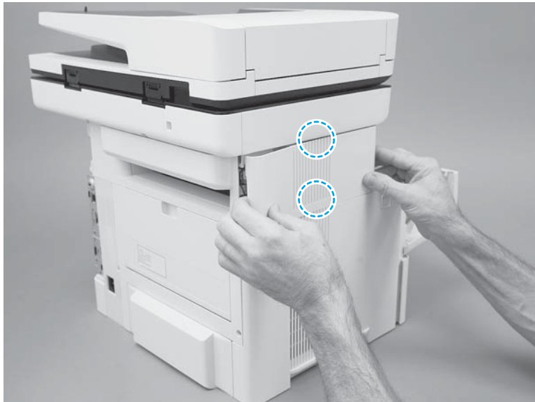
Figure 1-458 Engage two tabs
