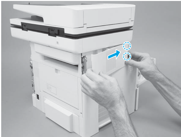
Figure 1-197 Slide the cover
