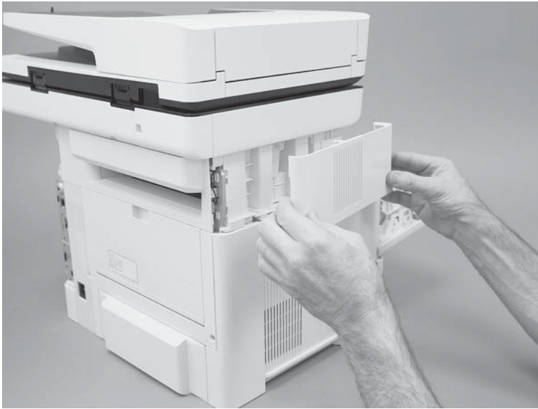
Figure 1-1709 Remove the cover
