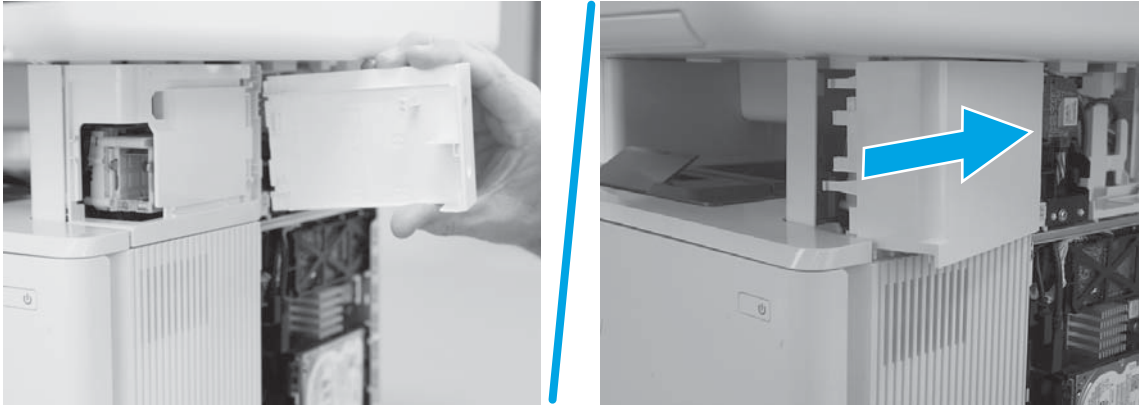
Figure 1-341 Install the door or cover
