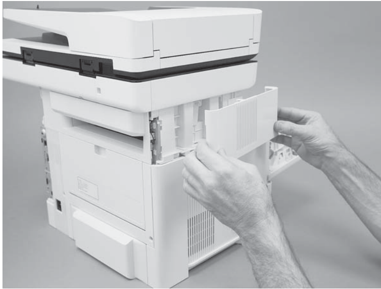
Figure 1-1174 Remove the cover
