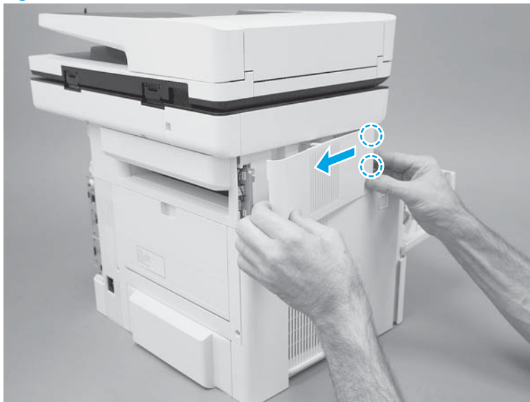
Figure 1-1375 Slide the cover
