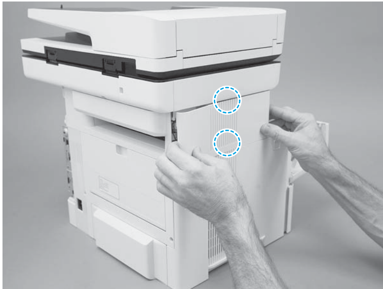
Figure 1-1654 Engage two tabs
