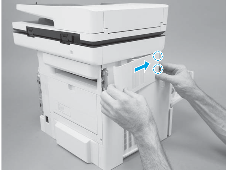
Figure 1-457 Slide the cover
