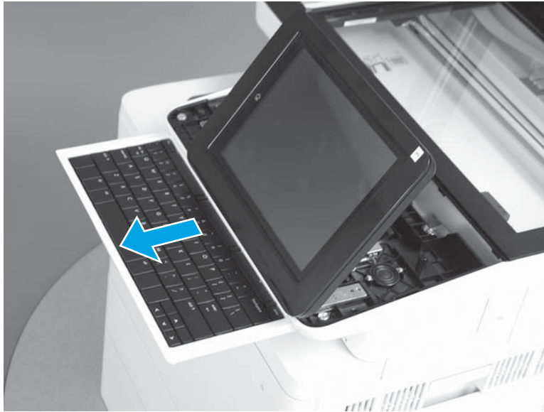
Figure 1-108 Slide the tray out
