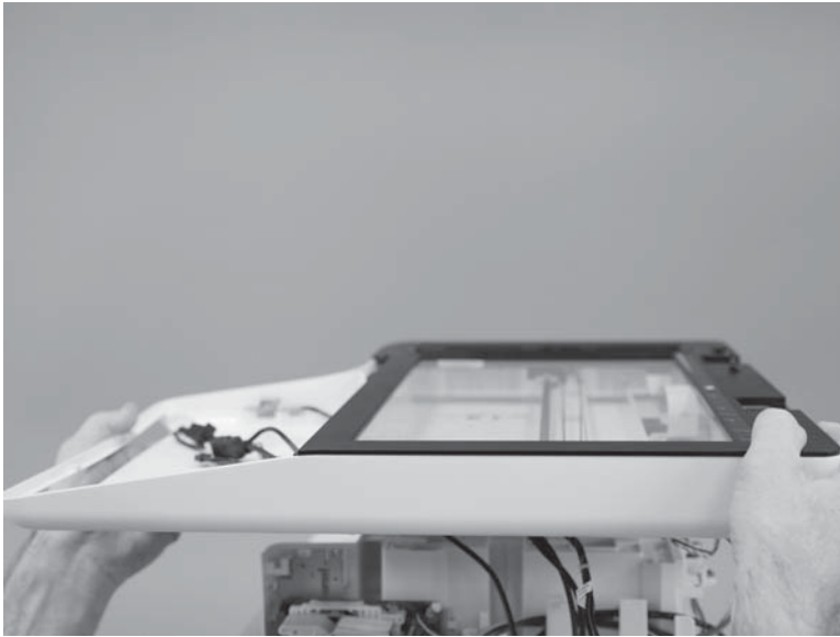
Figure 1-738 Remove the SSA
