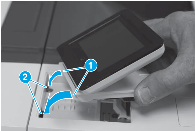
Figure 1-1678 Install the control panel
