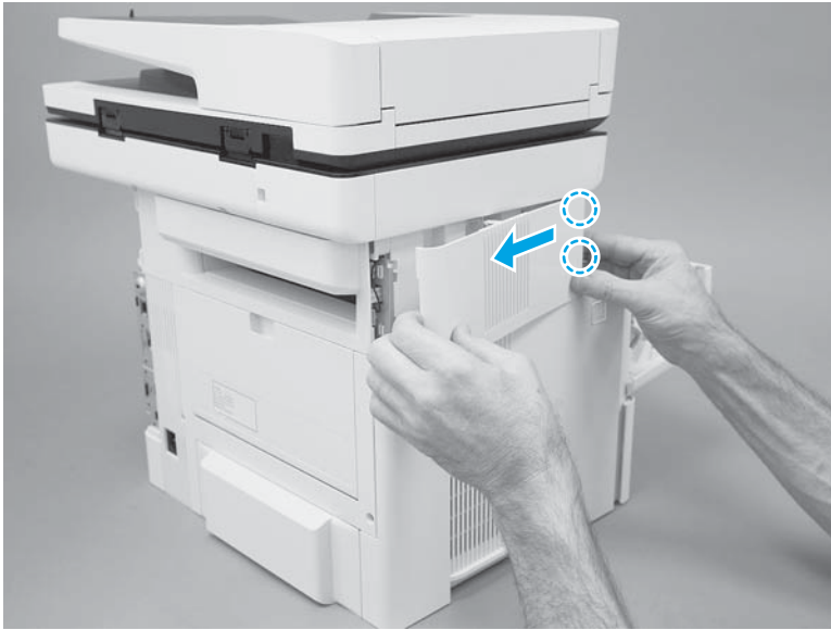
Figure 1-203 Slide the cover
