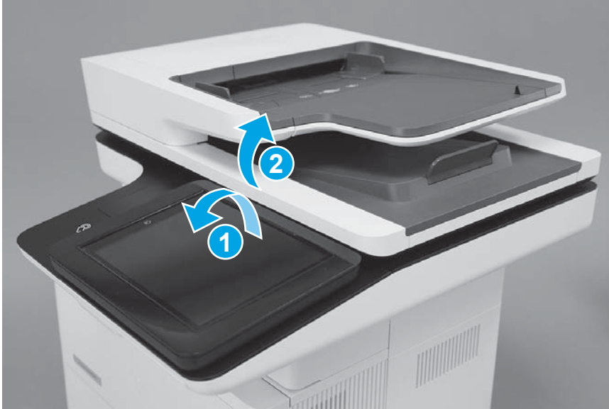
Figure 1-168 Open the document feeder
