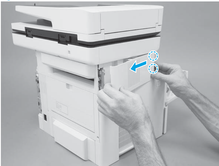
Figure 1-1173 Slide the cover
