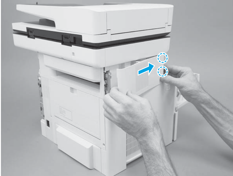
Figure 1-1485 Slide the cover
