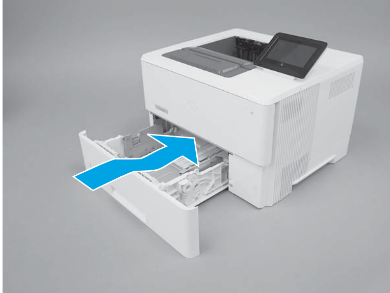
Figure 1-473 Install the tray
