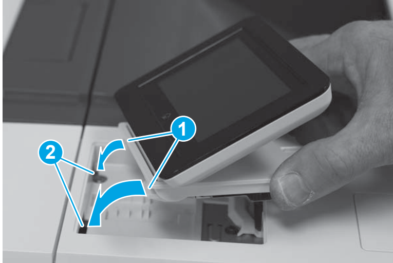
Figure 1-550 Install the control panel
