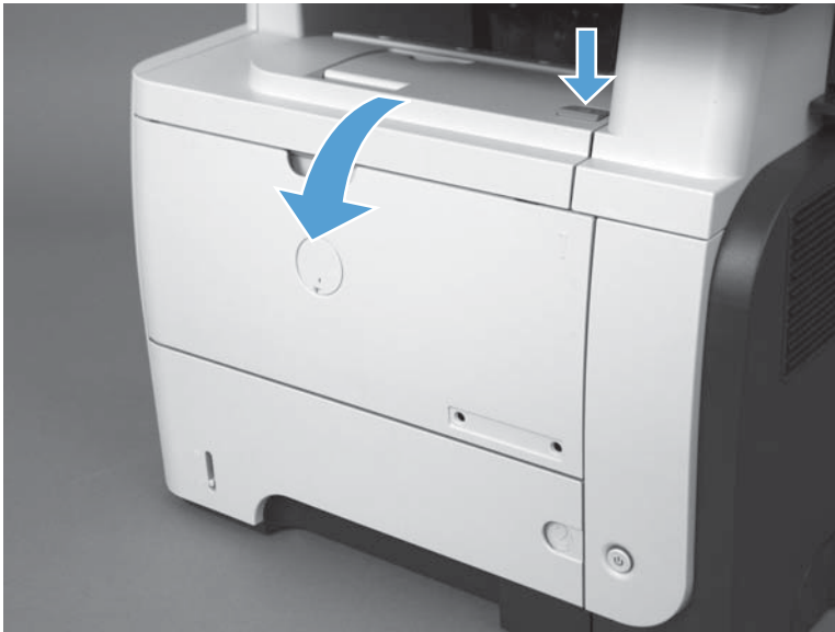
Figure 1-7 Remove the toner cartridge (1 of 2)
