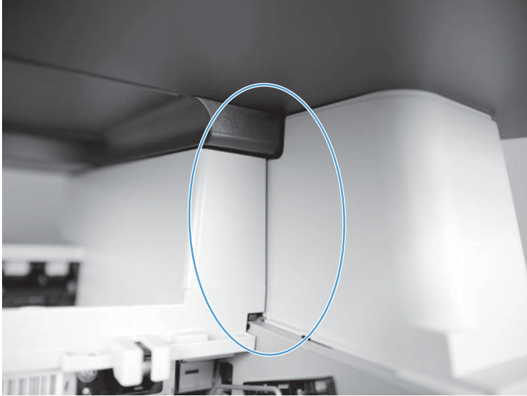
Figure 1-151 Reinstall the right cover assembly: incorrect alignment
