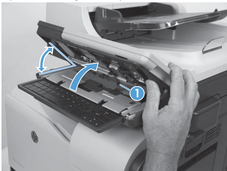
Figure 1-18 Raising the control panel to access the FFC connector (1 of 2)
