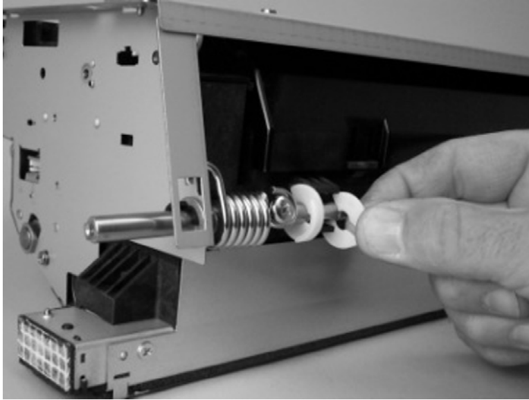
Figure 6-49 Remove the ADF optical assembly (4 of 13)
