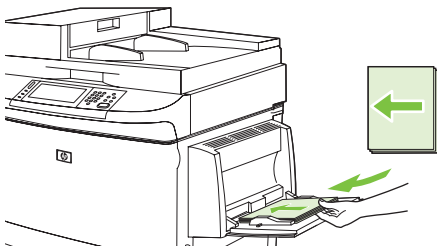
Figure 3-2 Load Tray 1 (2 of 3)
