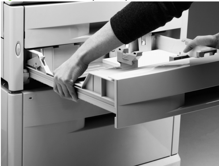
Figure 6-155 Remove Tray 2 or Tray 3
