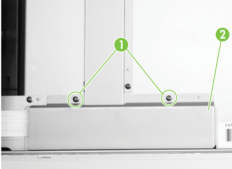
Figure 6-116 Remove the flatbed intermediate PCA (1 of 2)
