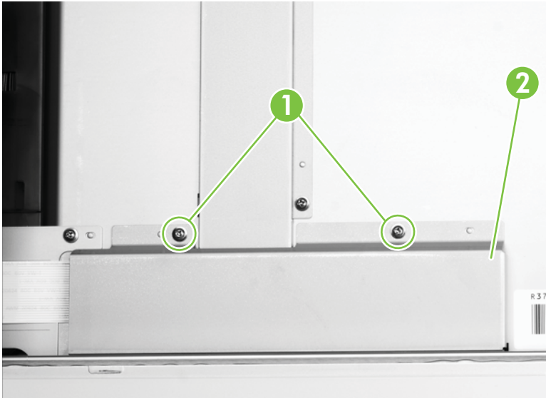
Figure 6-63 Remove the flatbed optical unit (1 of 6)
