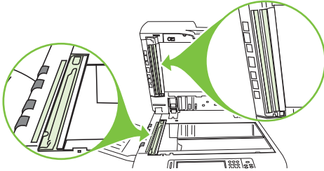
Figure 4-9 Clean the ADF delivery system (2 of 5)
