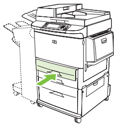
Figure 7-29 Clear jams in Trays 2 and 3 (2 of 3)
