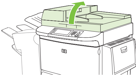
Figure 4-8 Clean the ADF delivery system (1 of 5)
