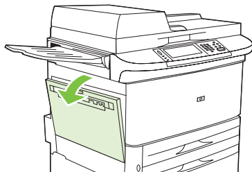
Figure 7-78 Clear jams in the left door (2 of 4)
