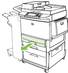
Figure 3-10 Load undetectable standard-size paper in Trays 2, 3, and 4 (1 of 6)
