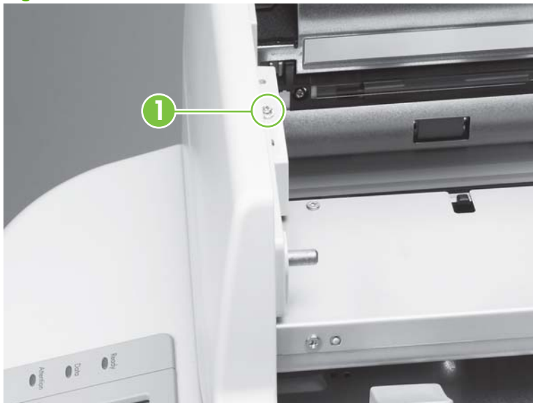
Figure 6-13 Remove the ADF front cover
