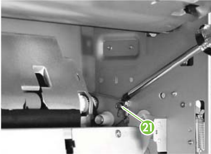
Figure 6-101 Remove the lower registration roller assembly (11 of 11)
