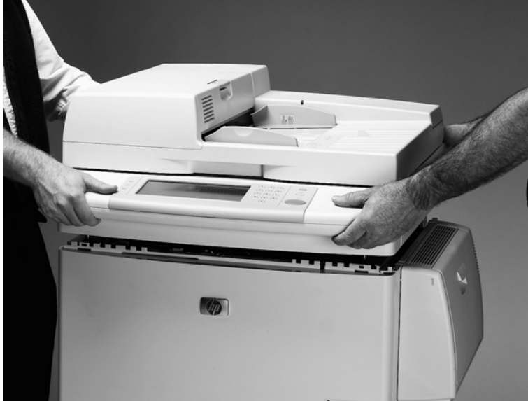
Figure 6-129 Remove the scan engine (6 of 7)
