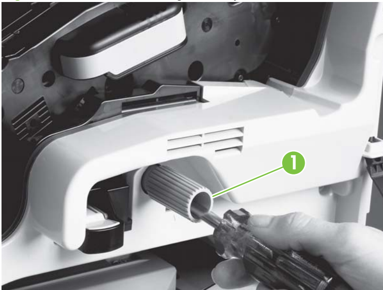
Figure 6-158 Remove the registration-jam-removal knob
