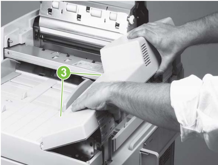
Figure 6-12 Remove the ADF back cover (2 of 2)
