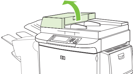
Figure 4-20 Clean the ADF rollers (4 of 6)
