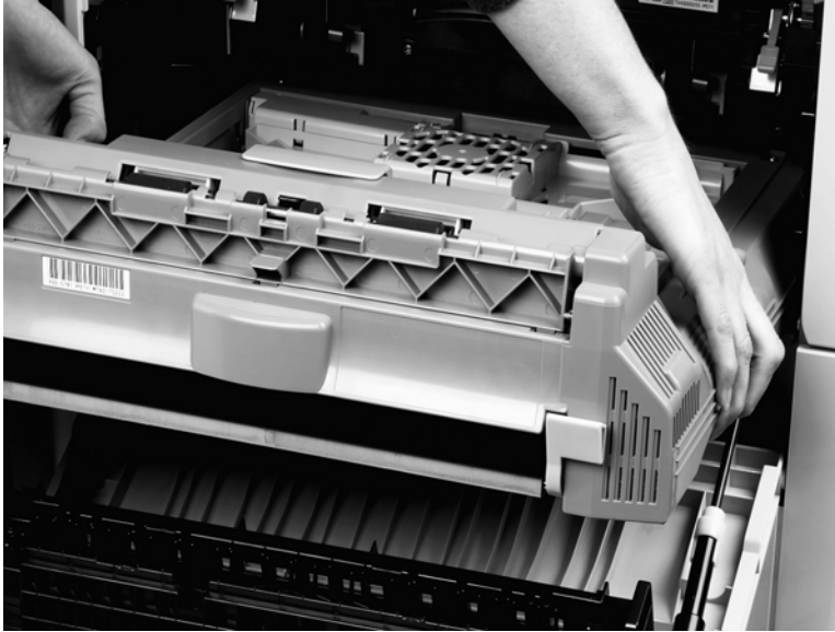
Figure 6-171 Remove the duplexer (2 of 2)
