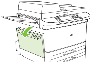
Figure 7-18 Clear jams in the duplex printing accessory (2 of 6)
