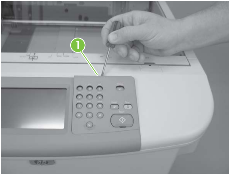
Figure 6-3 Remove the control panel (1 of 3)
