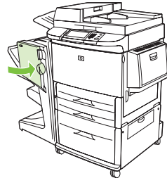
Figure 7-66 Clear a staple jam from the multifunction finisher (11 of 11)
