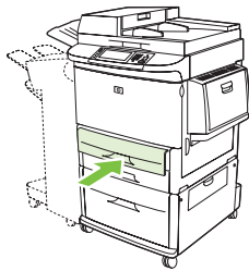
Figure 3-21 Load custom media in Trays 2, 3, and 4 (6 of 6)
