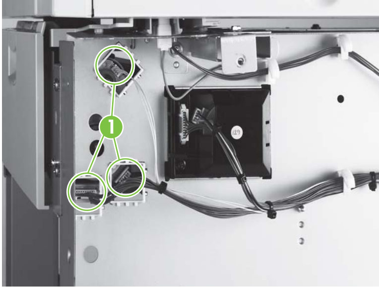
Figure 6-205 Remove the registration assembly (1 of 2)
